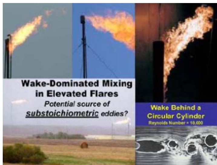
Figure 7 - Effect of crosswind on flame stability [13]
