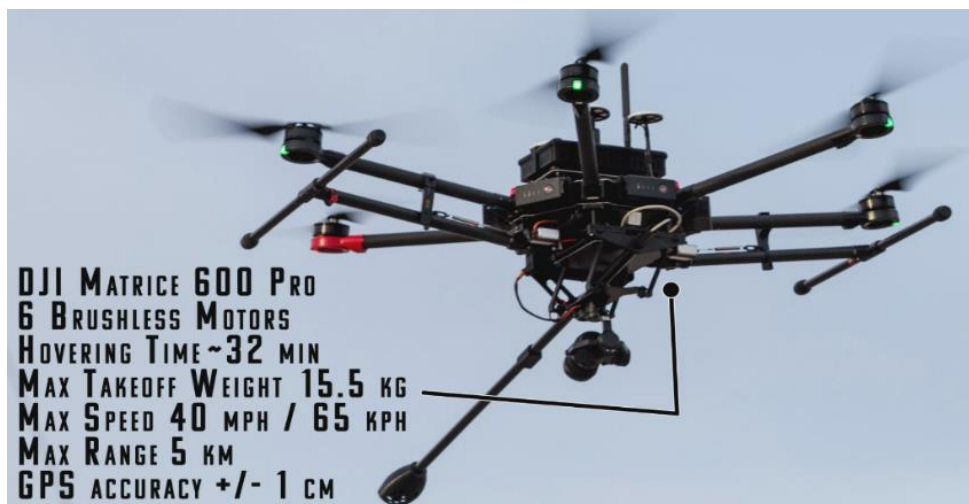
Figure 10 - EAGLE system mounted on a DJI UAS platform
