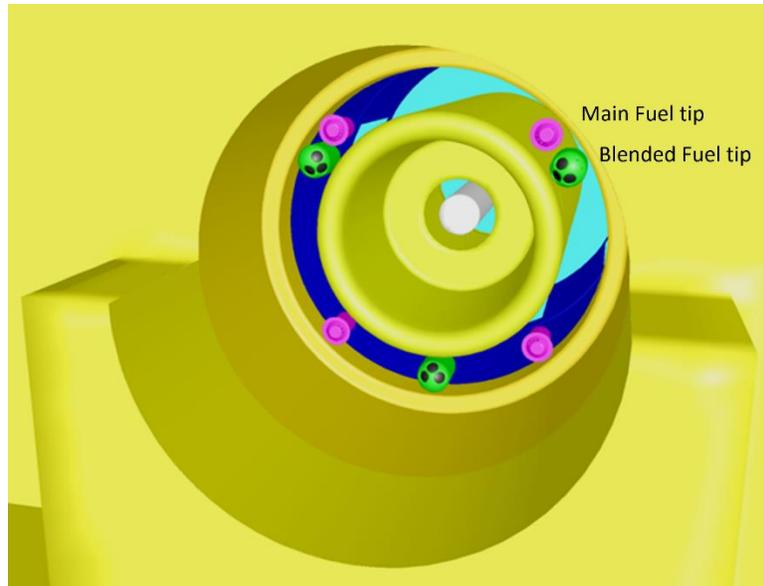
Figure 2 - Multi-fuel burner with main fuel tips (purple) and blended fuel tips (green)
