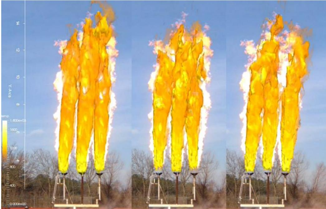
Figure 11 – Comparison of Predicted and Measured Flame Shape for an ethylene combustion test (predicted flame image overlaid to measured flame image)
