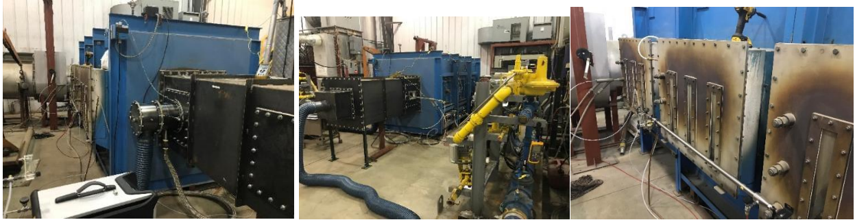
Figure 3: Design I burner (left) and cross air flow mixing chamber installed on the GTI test furnace (left, center) and Sideview of test furnace with emissions sampling probe installed at the far end (right)
