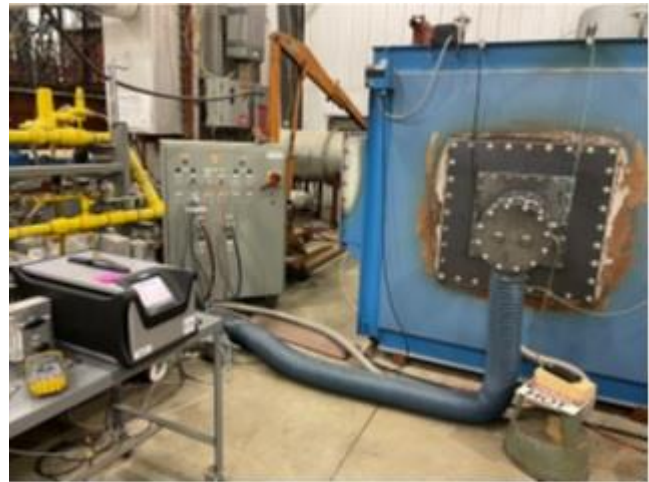
Figure 4: Setup for tests without cross air flow firing directly inside the furnace
