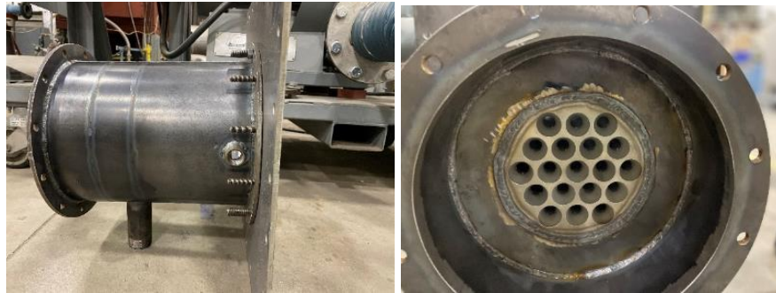
Figure 9: Sideview and combustion air inlet ends of the fabricated Design II burner section housing the nozzle assembly
