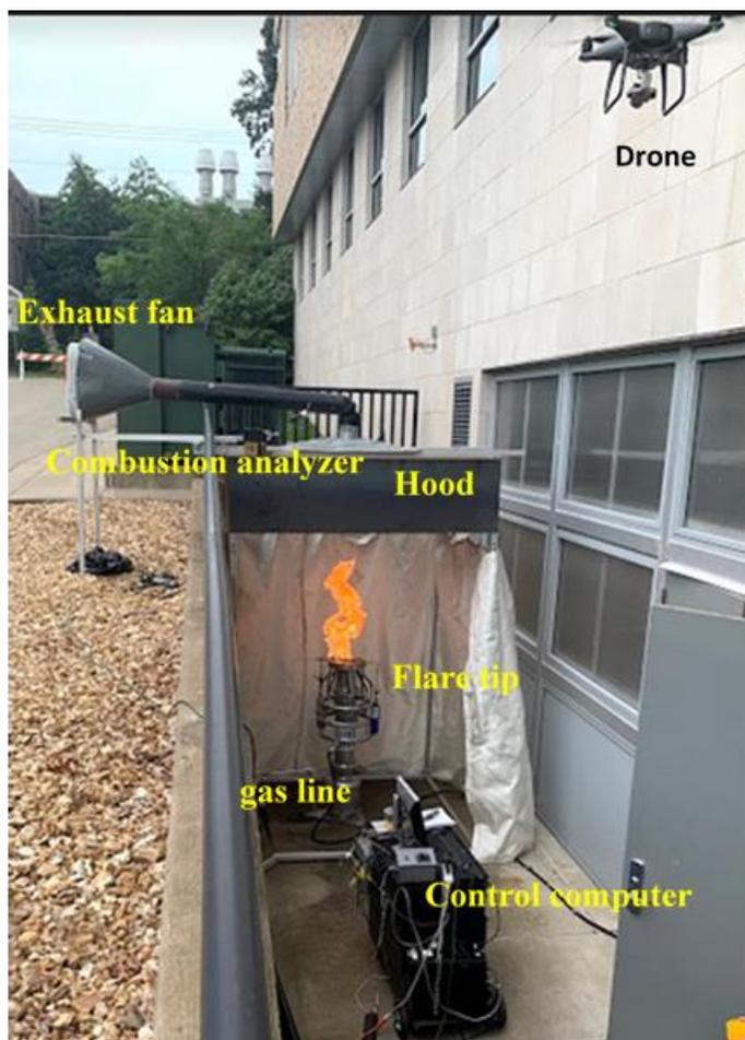
Figure 2 - Flare Test Setup
