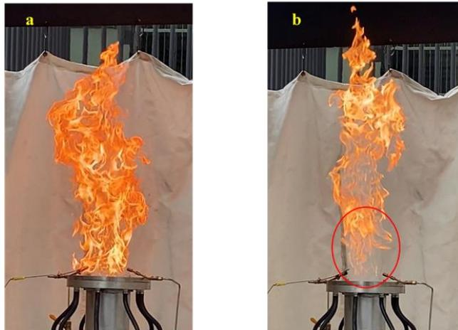
Figure 4 - Flame above Flare Tip with 20 L/min propane with: a) 0 cfm assist air, b) 8 cfm assist air
