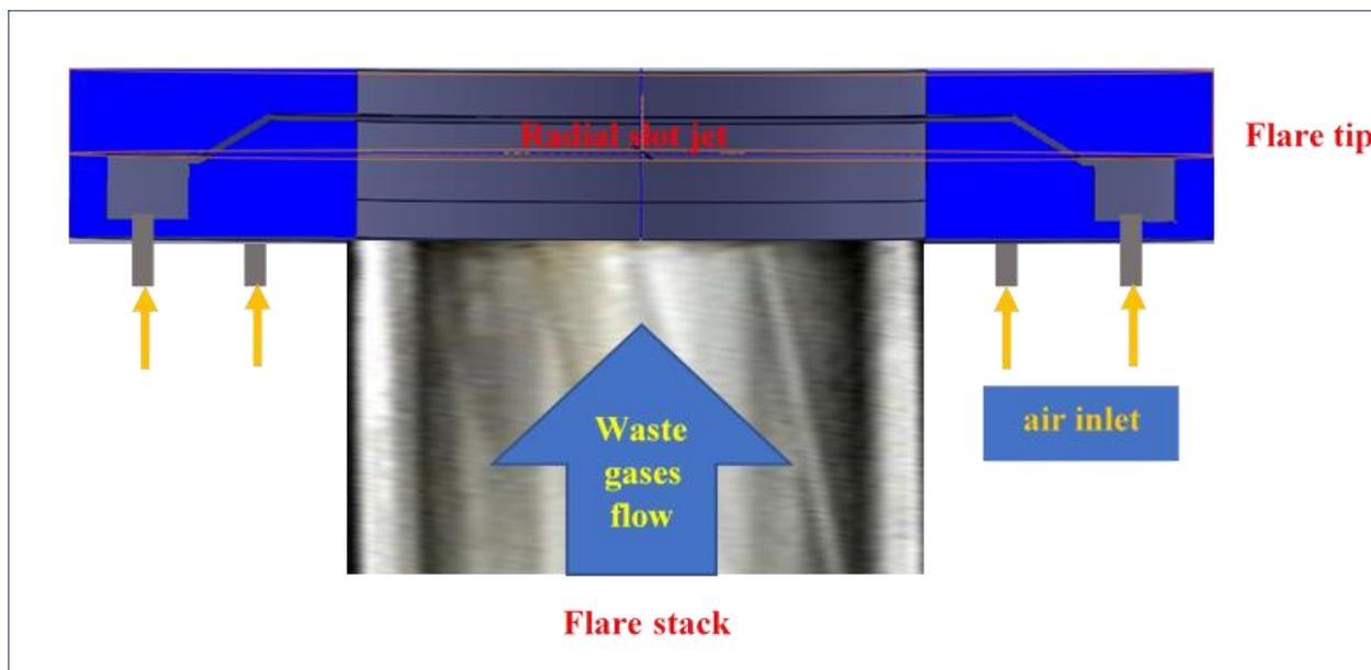
Figure 1 – Aero-nozzle flare tip design
