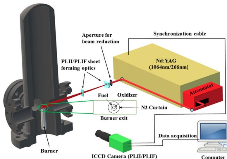
**Figure 1.** A high-pressure high-temperature experimental vessel with a burner in place along with a laser maneuvered through a series of lenses and mirrors.
