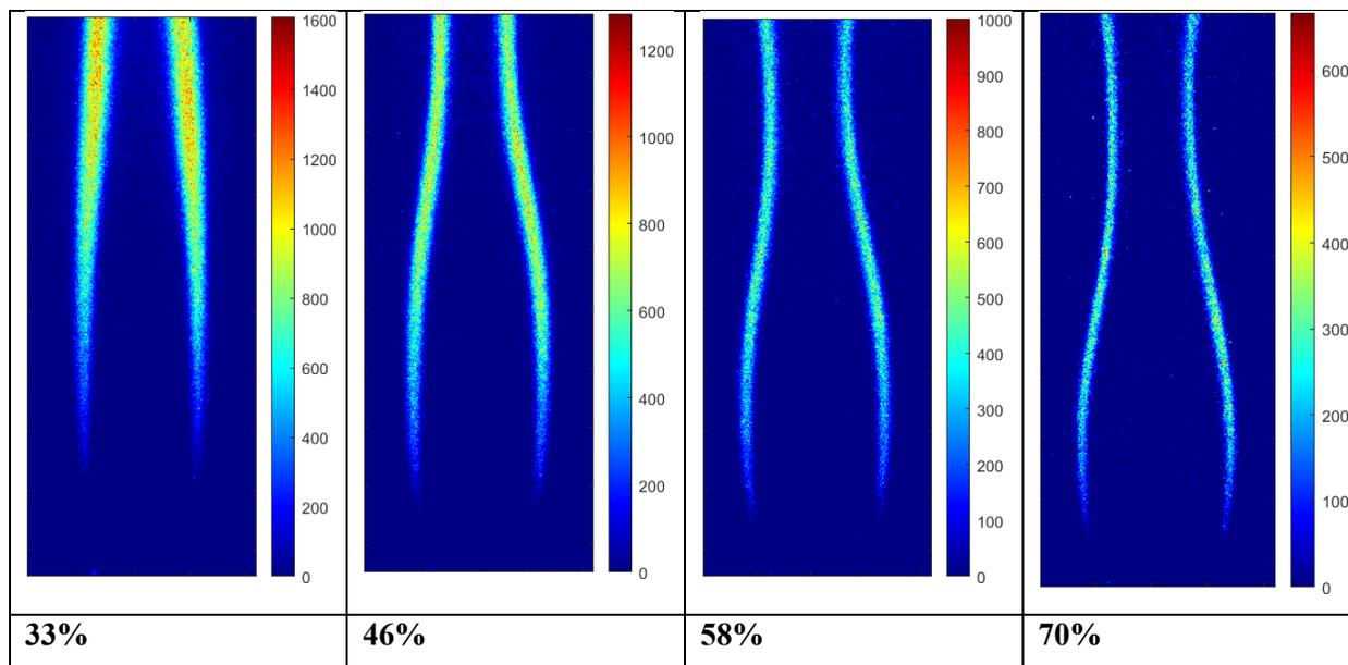
**Figure 4.** Raw LII images for flames with different O<sub>2</sub> concentrations in oxidizer steam at 4 bar. Laser crosses the flame from the right to the left side (Individual color legend is presented for each image).
