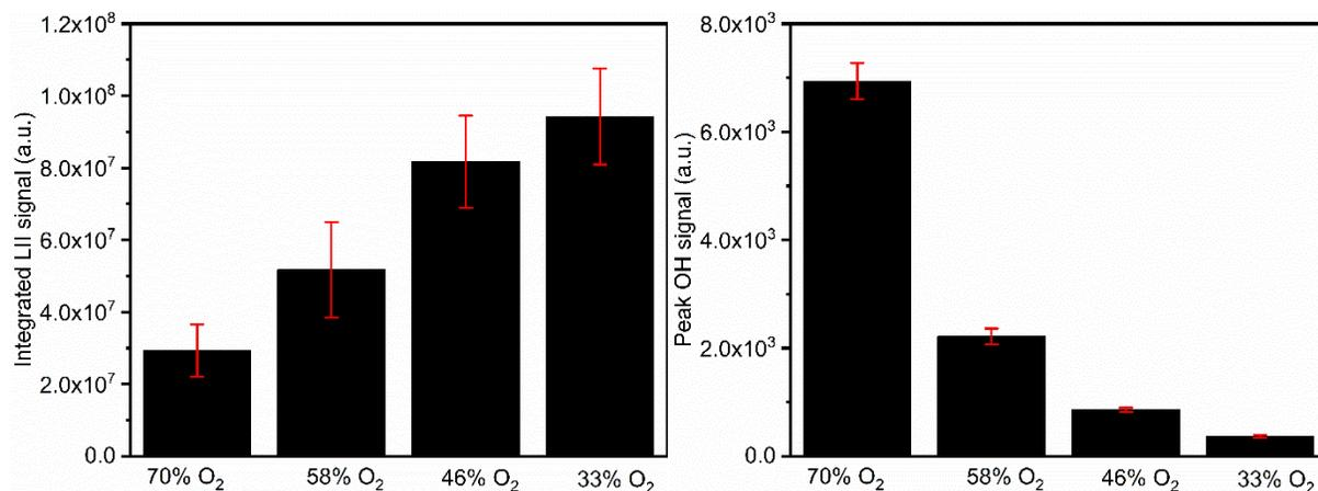
**Figure 6.** (a) Integrated LII intensity vs O<sub>2</sub> concentration at 4 bar. (b) Peak OH\* intensity vs O<sub>2</sub> concentration at 4 bar.
