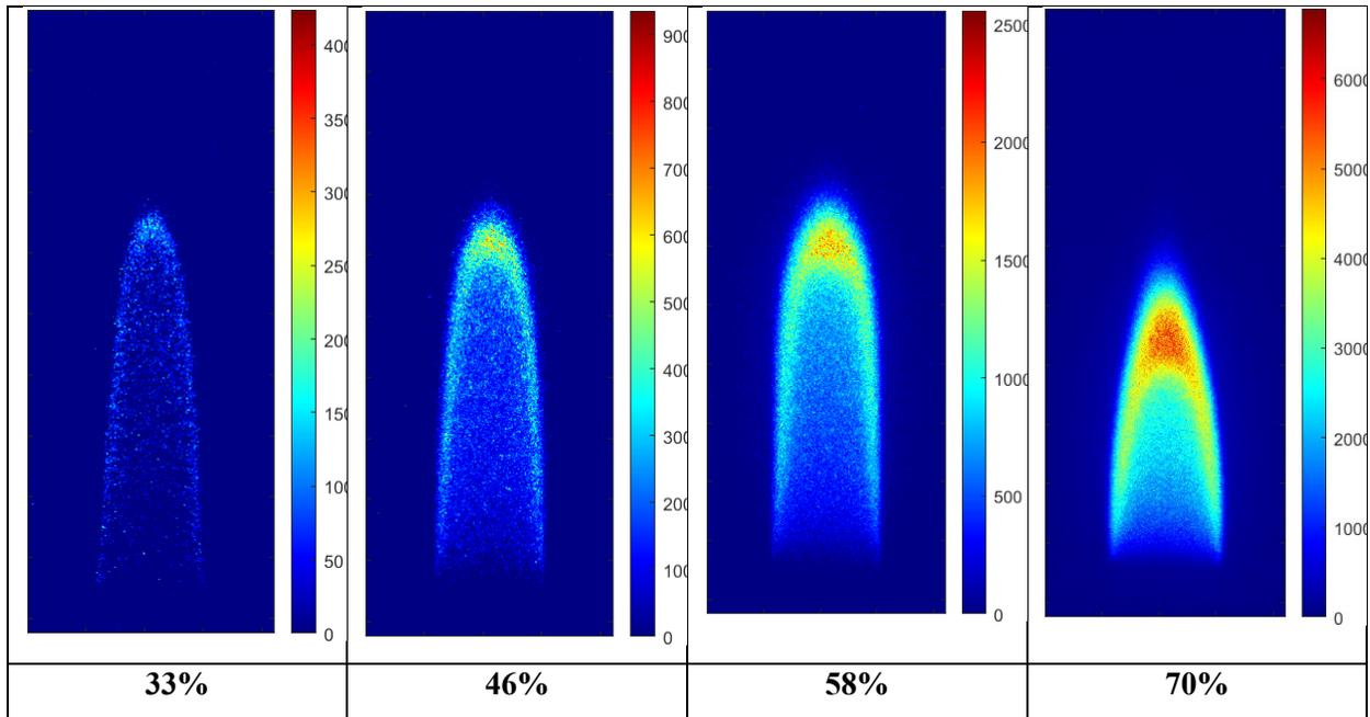
**Figure 3.** OH\* intensity signal at 4 bar, illustrating the effect of O<sub>2</sub> concentration on the flame structure. The individual color legend is presented for each image.
