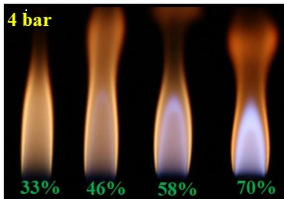
**Figure 2.** Images for flames with different O<sub>2</sub> concentrations in oxidizer steam.
