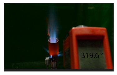
Figure 7 Thermal testing showing the temperature measurement of the ClearSign EYE probes at the location indicated by the two red dots.
