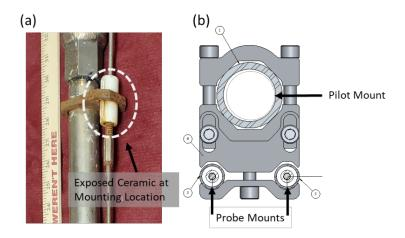
Figure 5 Mounting configuration for (a) flame rods and (b) ClearSign EYE
