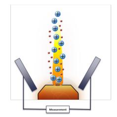
Figure 1 Flame detection using two capacitively coupled probes
