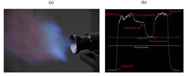
Figure 3 (a) Proof of concept burner firing, (b) Example output measurements showing the capability of high-resolution measurement of ion concentrations within the flame.
