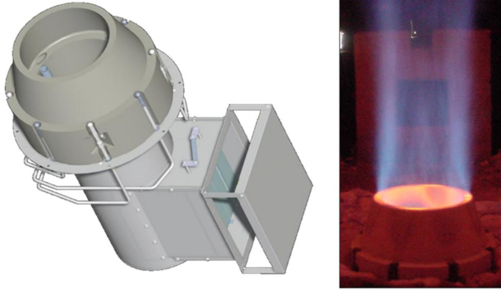
Figure 9 Burner with a round tile.
