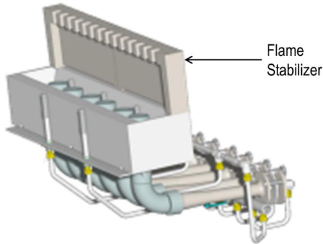
Figure 7 Burner tile with a “teeth” for flame stabilization.
