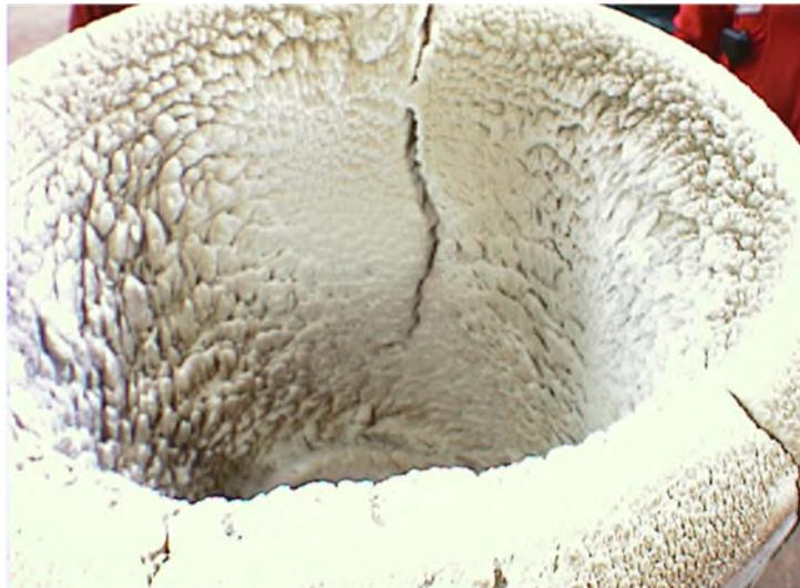
Figure 20 Catalyst build-up on a regen tile.
