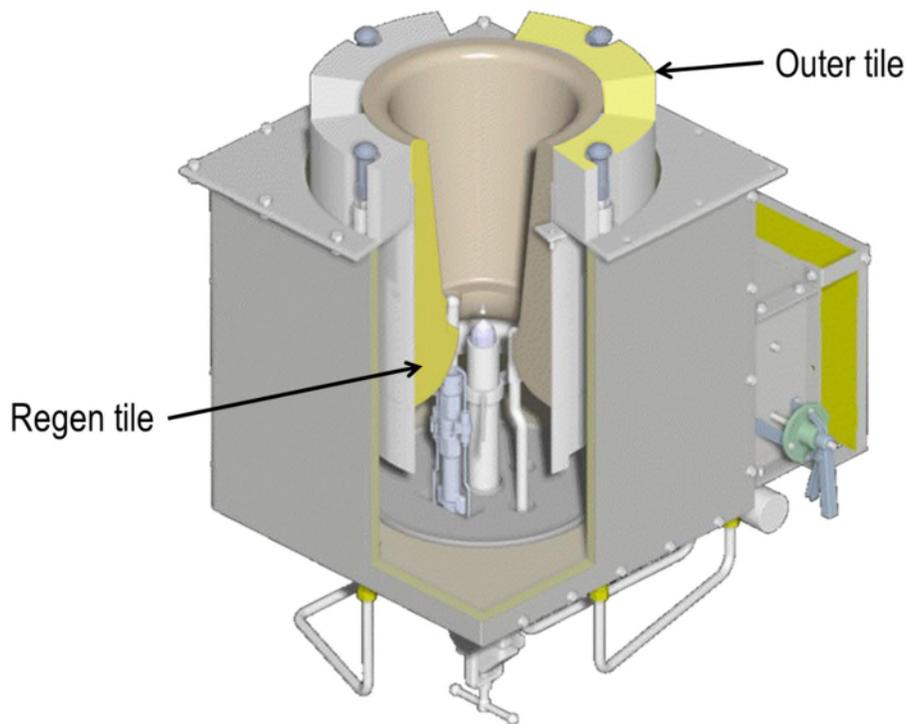
Figure 8 Example of an inner regen tile for a combination burner capable of firing on gas or liquid fuel.
