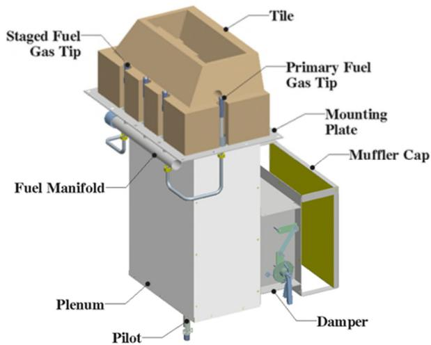
Figure 10 Burner with a rectangular tile.
