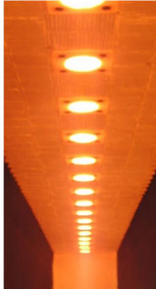
Figure 2 Downfired burners in a reformer furnace.
