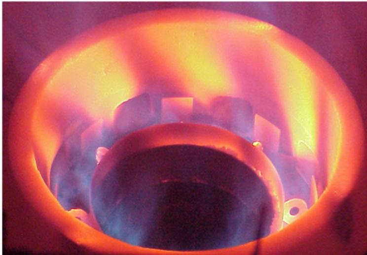
Figure 5 Burner tile with angled holes to produce swirl.
