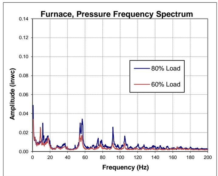
Figure 13 – Furnace Pressure-Processed (Case Study)
