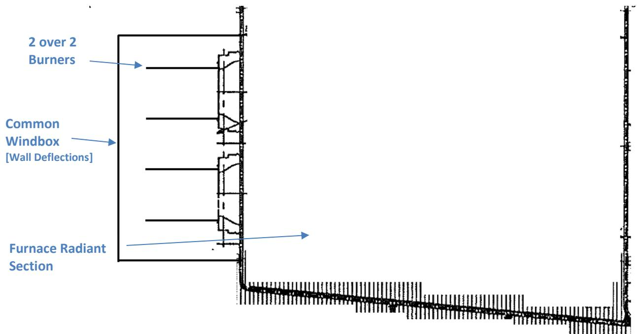
*Figure 8 – Large Field-Erect Furnace Cross-section*
