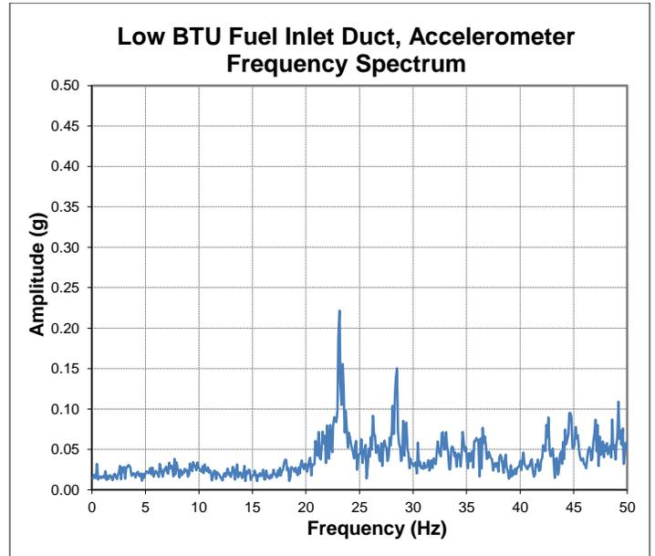
Figure 17 – Low BTU Fuel Supply Duct Acceleration-Processed
