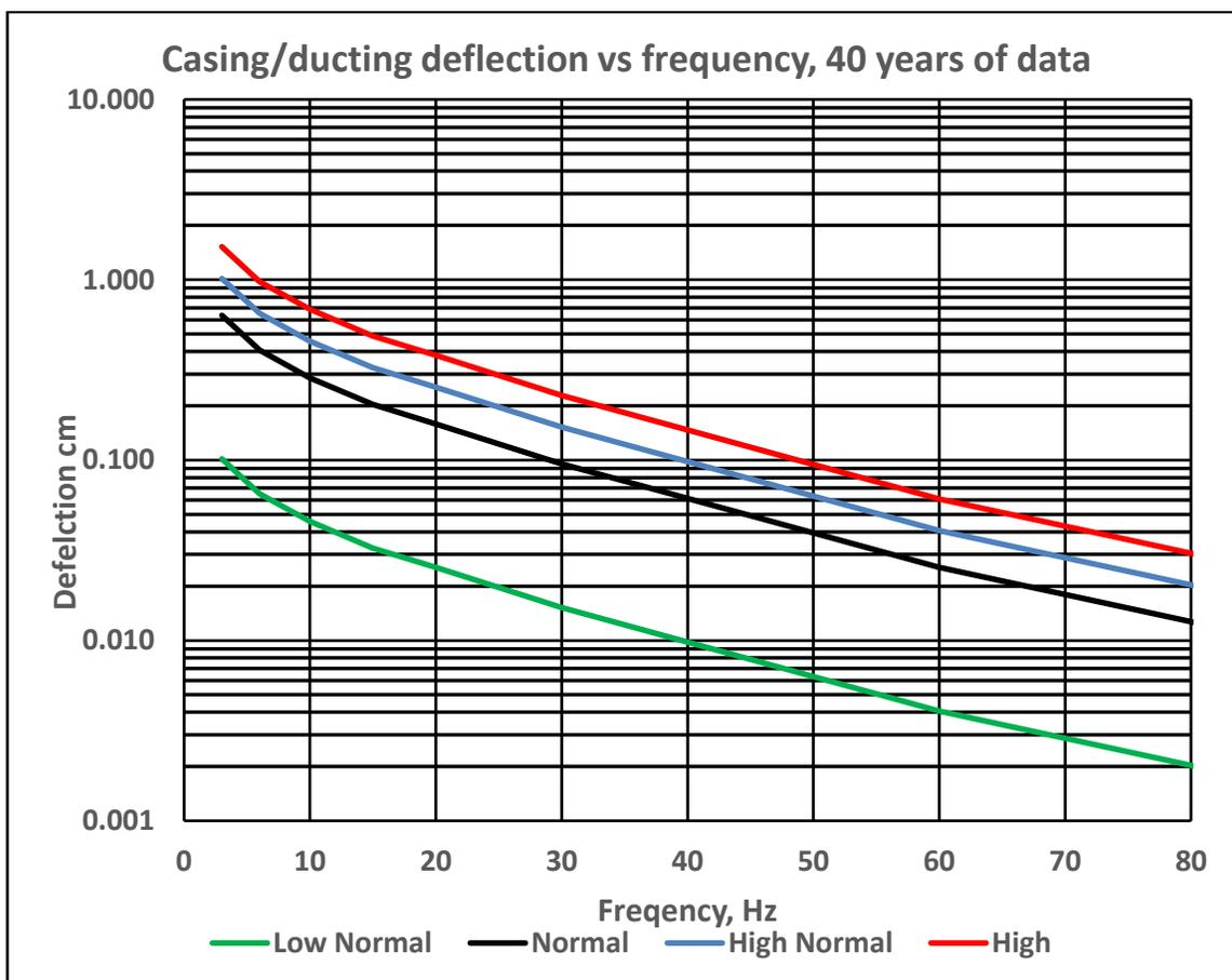
Figure 1 – Observed casing and ducting deflections based on site problems and expert perception
