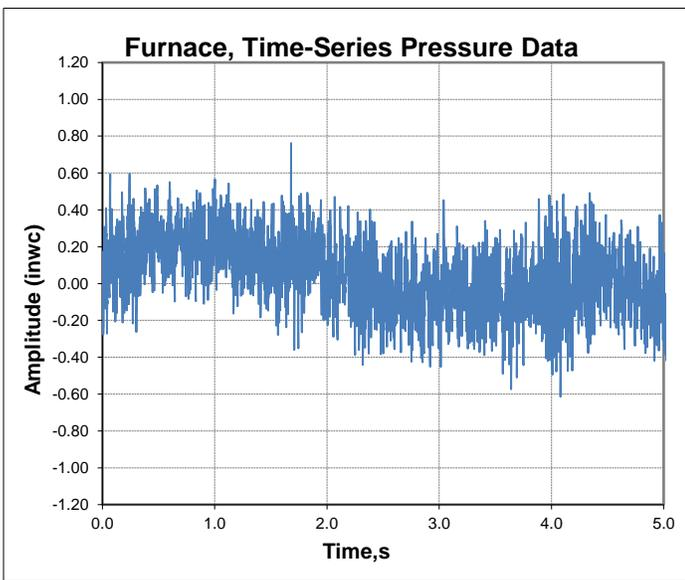
Figure 12 – Furnace Pressure-Raw (Case Study)
