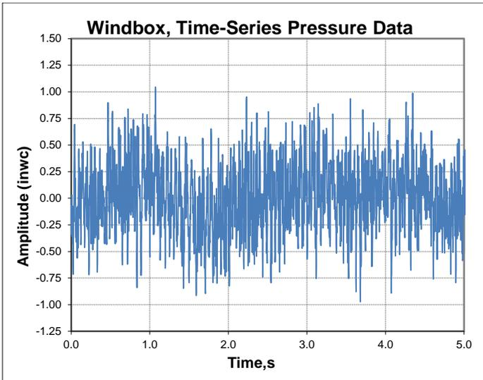
Figure 10 – Windbox Pressure-Raw (Case Study)
