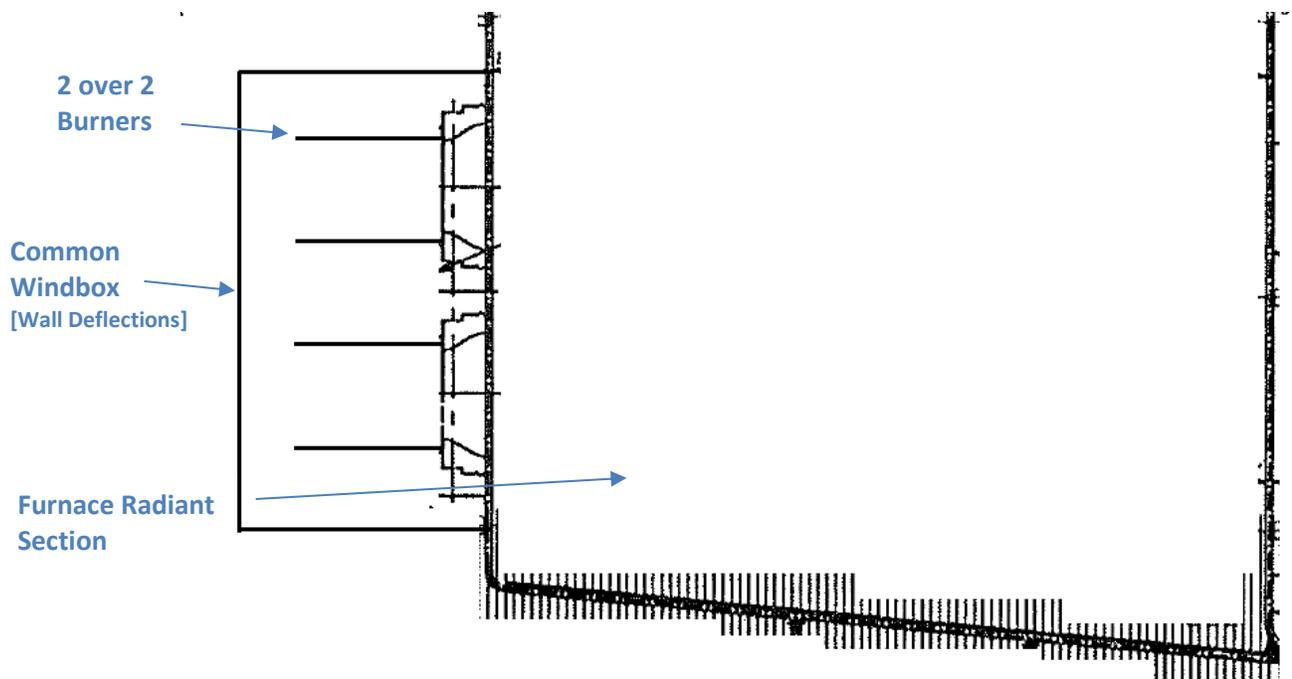
*Figure 8 – Large Field-Erect Furnace Cross-section*
