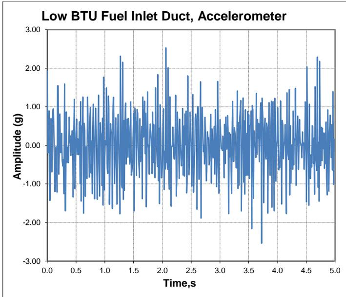
Figure 16 – Low BTU Fuel Supply Duct Acceleration-Raw
