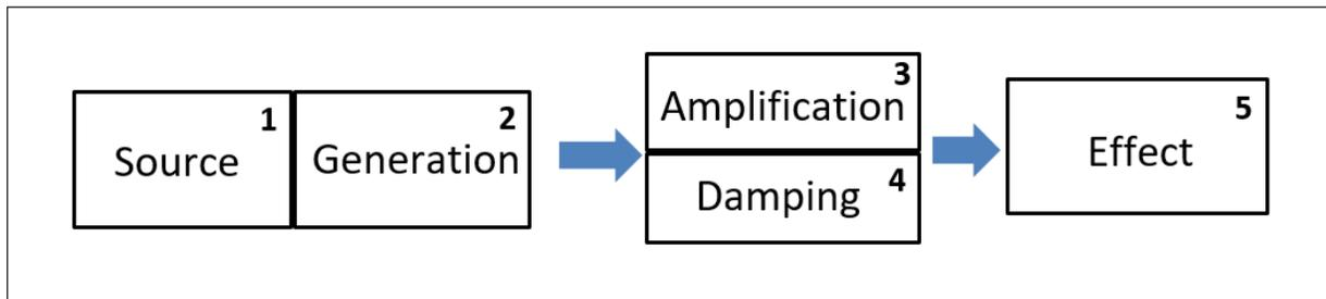
Figure 6 – Sound Generation Process (Simplified)
