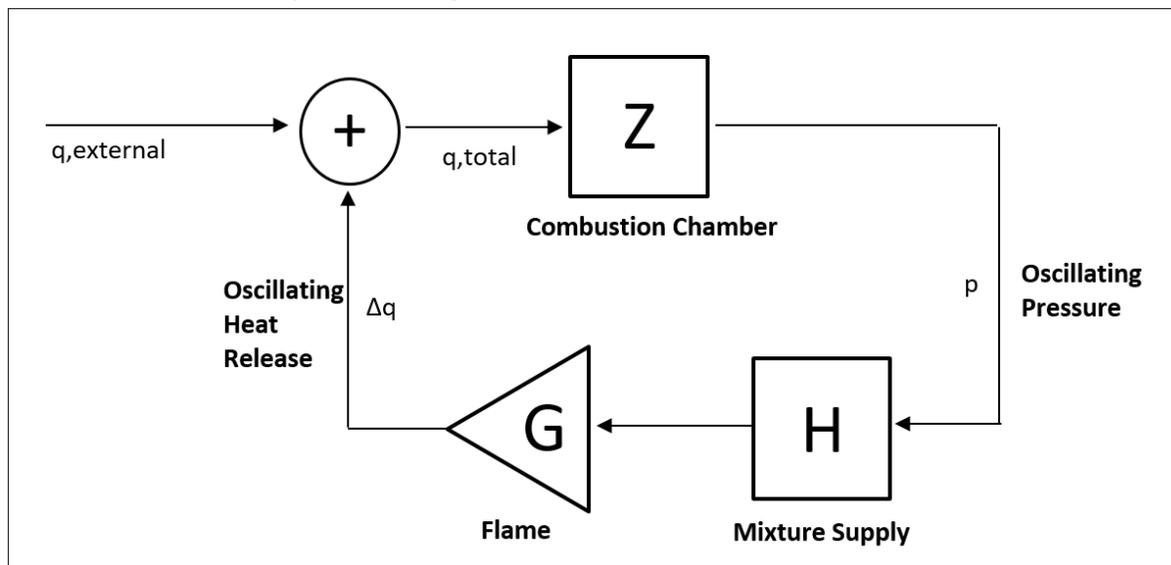
Figure 3 – Combustion Instability Feedback Loop Model [4]
