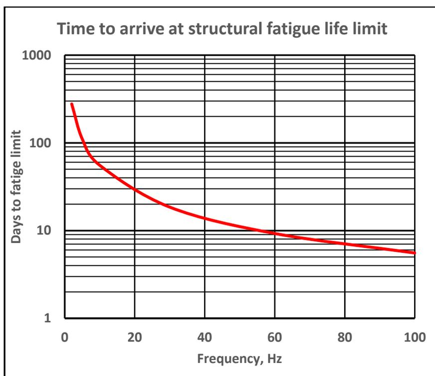
Figure 2 – Fatigue time limit vs vibration frequency [20]
