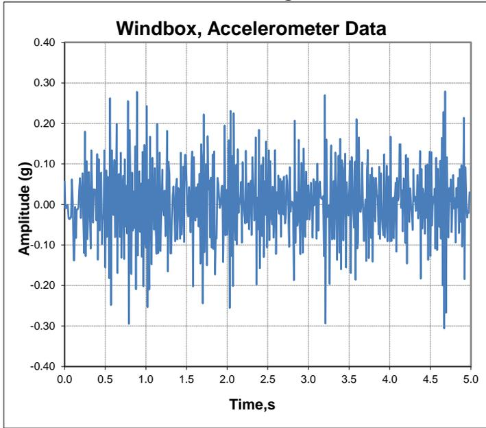
Figure 14 – Windbox Frontplate Acceleration-Raw
