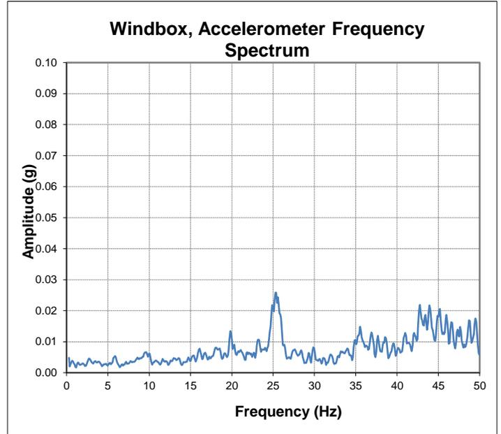
Figure 15 – Windbox Frontplate Acceleration-Processed
