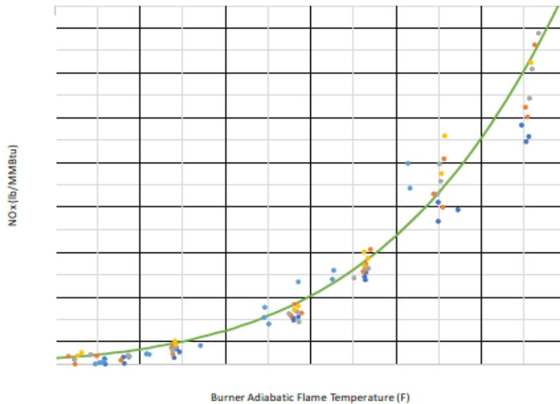
Figure 1: NOx levels as they relate to a burner adiabatic flame temperature.
