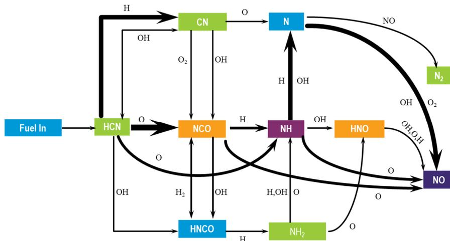
Figure 4: Expected nitrogen compound formations as considered in the Fenimore Mechanism.
