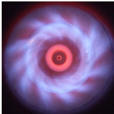
*Figure 3: Photo of an RMB burner in operation.*
