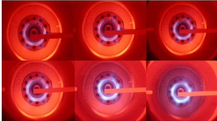
*Figure 2: Flame shape as adiabatic flame temperature increases.*
