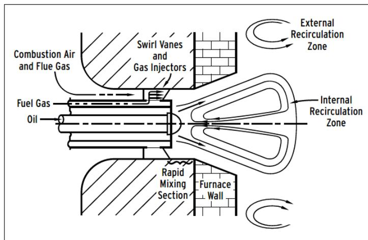
Figure 6: Demonstration of recirculation zones within the RMB burner.
