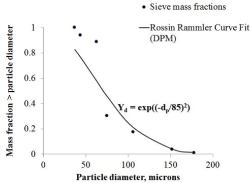
Figure 2: The Rosin-Rammler distribution function used to represent the PSD of the parent fuel.
