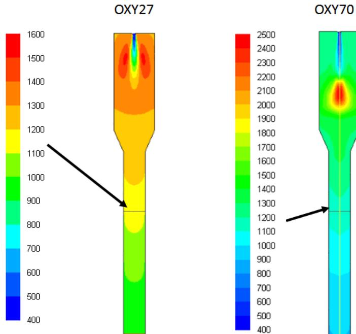
Figure 3: Predicted temperature contours in the OXY27 and OXY70 flames
