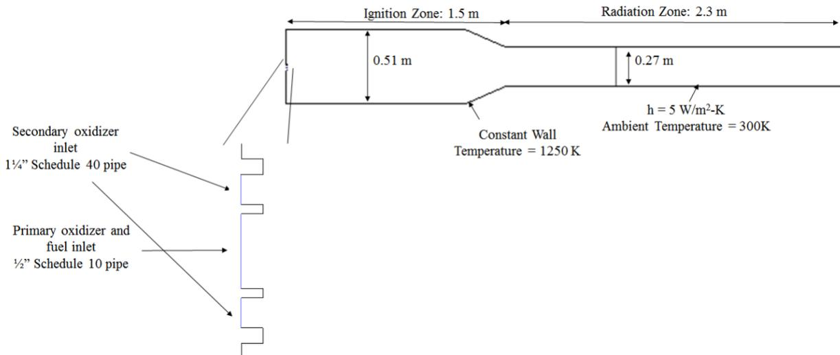
Figure 1: 2D, axisymmetric geometry designed to replicate the experimental 100 kW combustor.
