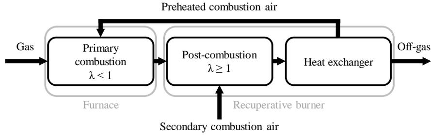
Figure 1: Concept for low scale reheating of semi-finished metal products [11]
