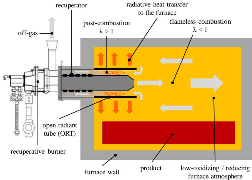
Figure 2: Concept of direct fuel rich firing and radiant tube heating [14, 15, 16]
