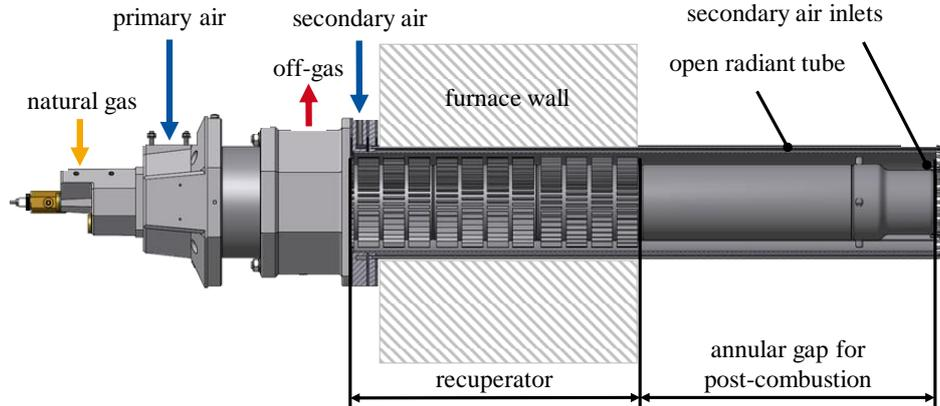
Figure 5: Cross section of the concept-burner [16]
