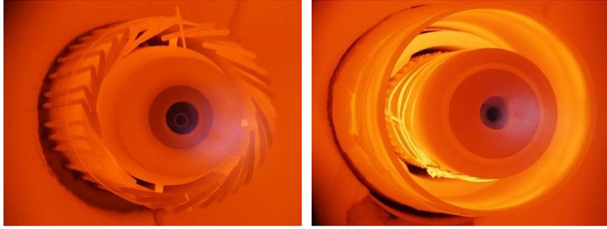
Figure 6: Picture of the concept-burner (left) and the ceramic prototype-burner (right) in a test furnace [14, 15]
