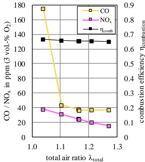
Figure 9: Measured off-gas emissions and thermal efficiency of the prototype-burner in configuration 1 [14, 19]
