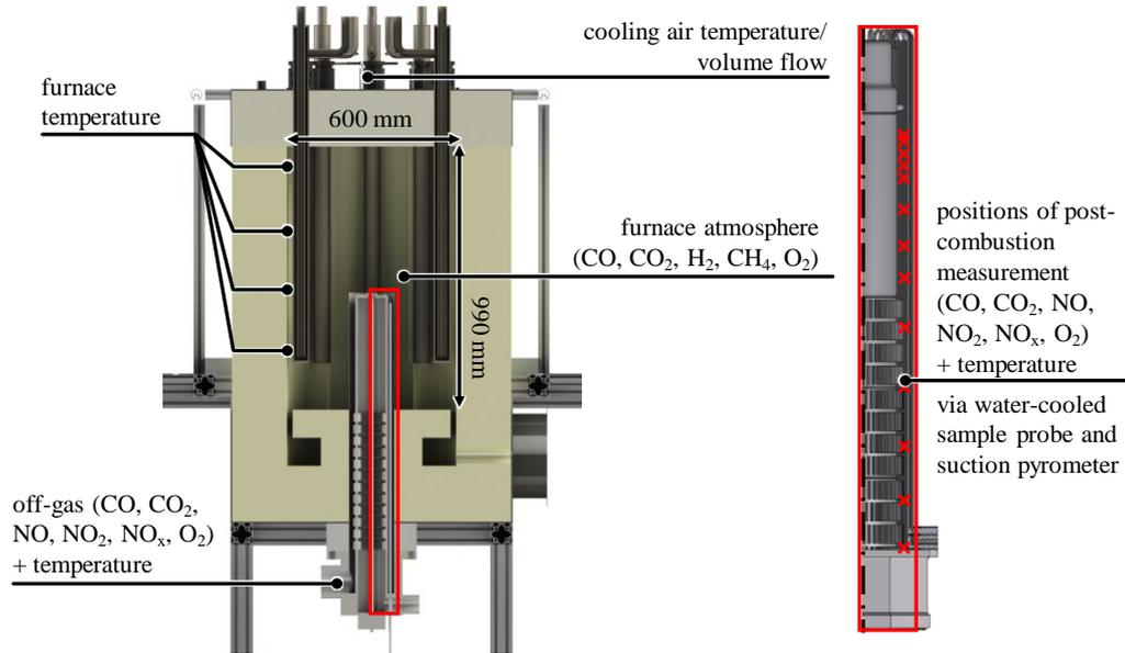
Figure 4: Experimental setup [19]
