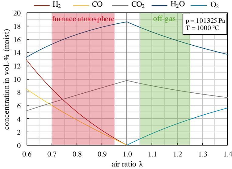
Figure 3: Operating range of the new burner [14]
