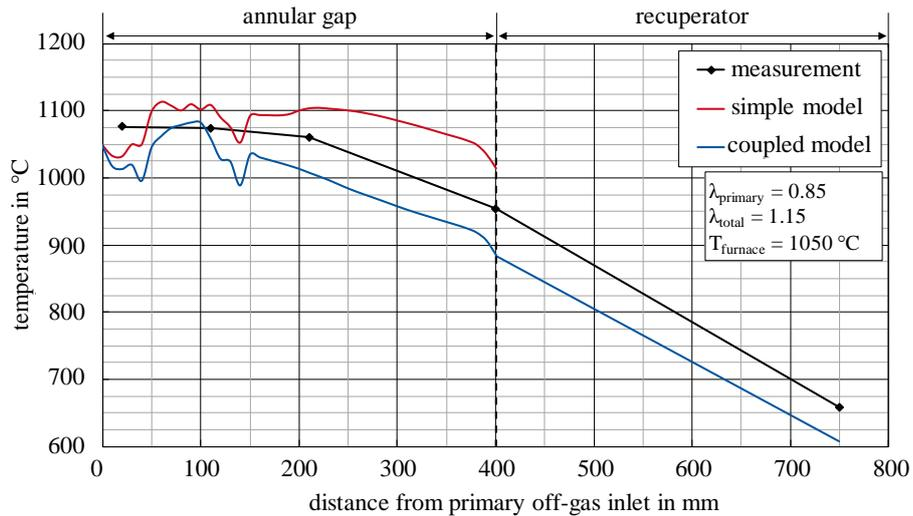
Figure 8: Temperature in the annular gap of the prototype-burner, burner configuration 2 [19]
