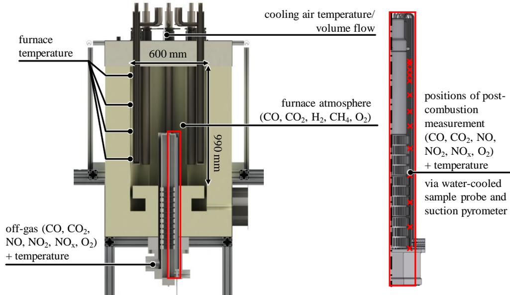
Figure 4: Experimental setup [19]
