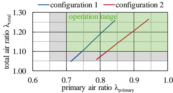
Figure 7: Operation range of the ceramic prototype-burner in a test furnace [14]
