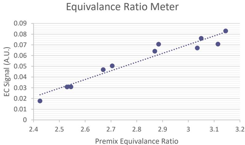
Figure 4 Calibration curve for equivalence ratio of burner.
