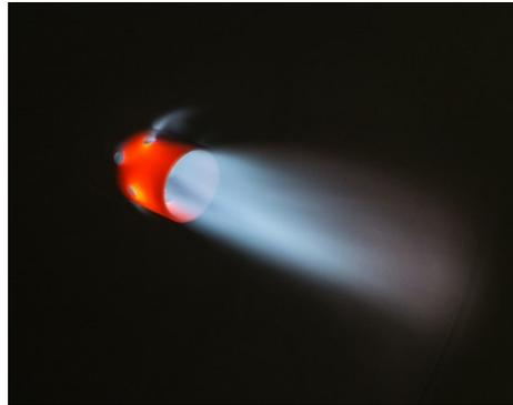
*Image 11: A properly operating pilot in an incinerator application.*
