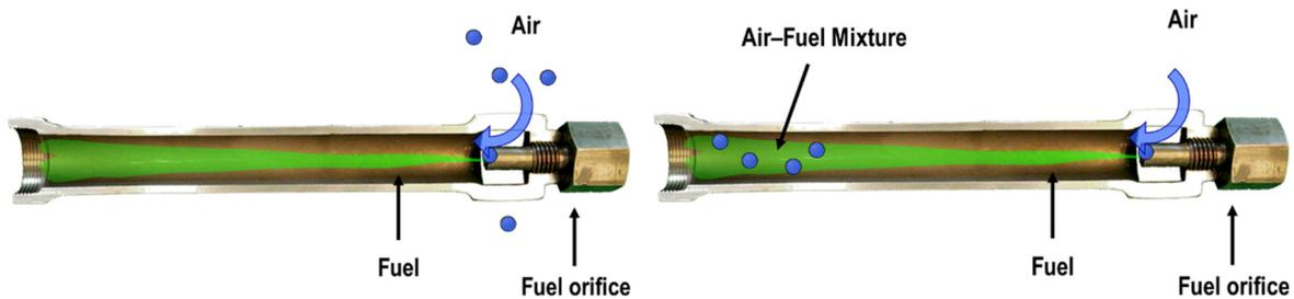
Image 4: Demonstration of how air/fuel mixer functions.
