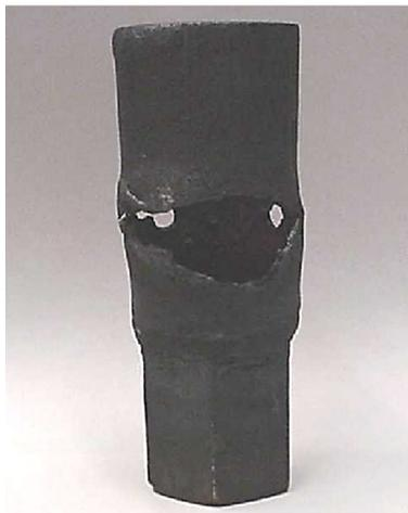
Image 10: Example of Damaged Pilot Tip
