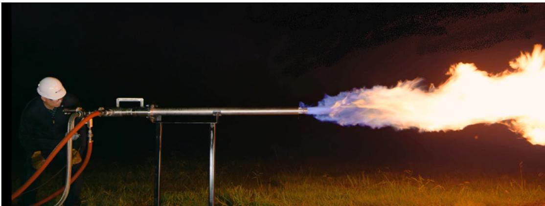
Image 9: Example of a high heat release pilot which can fire between 200,000 BTU/Hr to 20,000,000 BTU/Hr to cover a gap in heat control between a pilot and burner turndown
