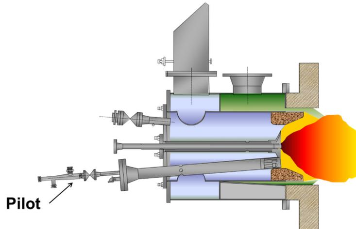
*Image 1: Typical pilot in an incinerator application.*
