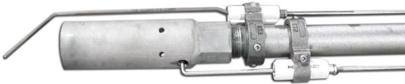
Image 5: Typical pilot assembly with high voltage igniter (lower portion) and flame rod for flame proving (upper portion).
