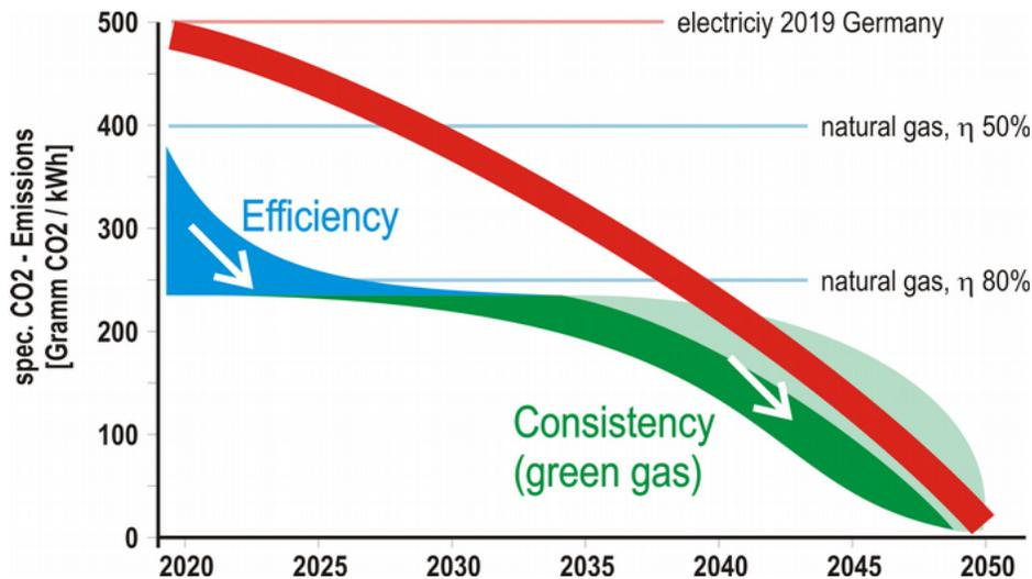
Figure 1: fossile CO<sub>2</sub>-emissions from high temperature process heating
