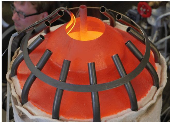
Figure 6: FLOX<sup>®</sup>-2 Burner
