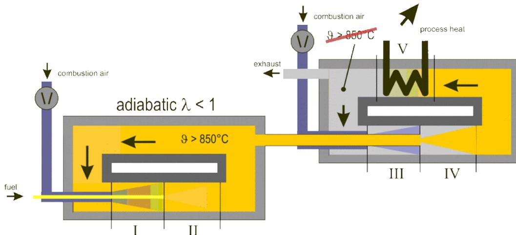
Figure 4: Two Stage Flameless Oxidation (FLOX®-2)
