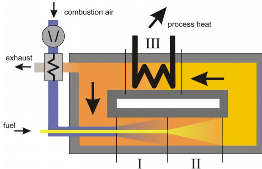
Figure 2: principle of Flameless Oxidation
