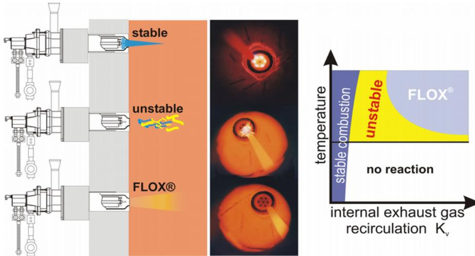
Figure 3: stable and unstable combustion
