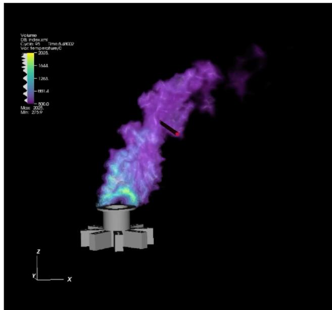
**Figure 3:** Volume rendered temperature with the red cylinder showing an example of the ID line-of-sight extraction from the LES data.
