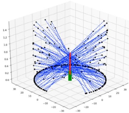
**Figure 7:** Example of the PFTIR instrument model sampling showing the variation in the targeting position and the wind direction effect. The flare stack is indicated with the green bar. The intersecting targets are shown with red dots. The starting and stopping locations of the PFTIR ray are indicated with black dots while the ray path is shown with the dashed blue line.
