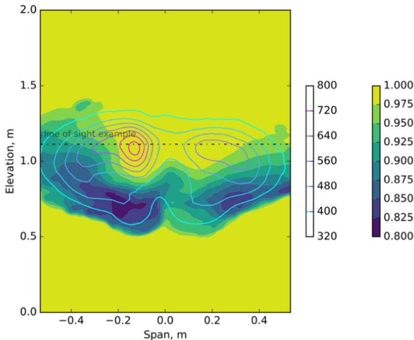
**Figure 5:** A two-dimensional filled contour plot of the combustion efficiency and line contour plot of temperature at the same downstream location.
