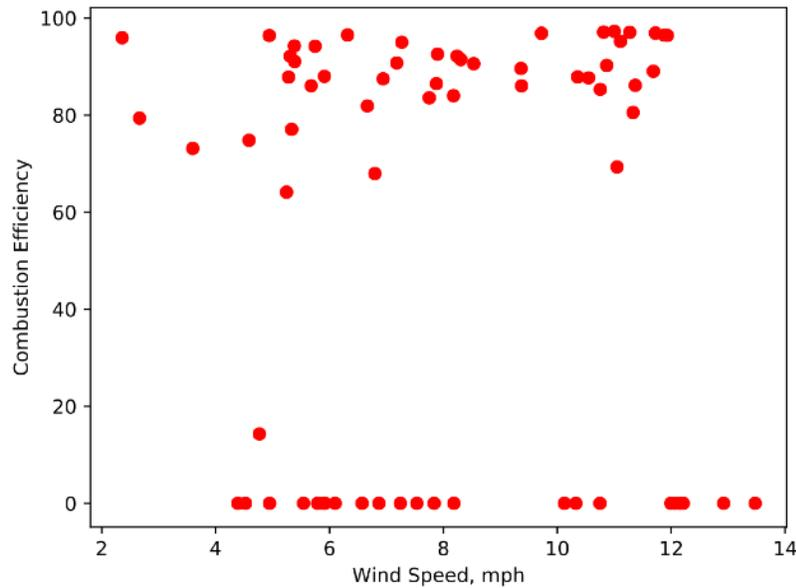
**Figure 2:** Measured combustion efficiency percentages as a function of the observed wind speed. Values at zero indicate failed readings.
