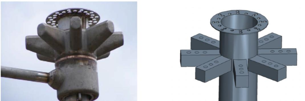
**Figure 1:** Image of the flare actual flare head (left) and the reconstructed geometry used in the LES simulation (right).
