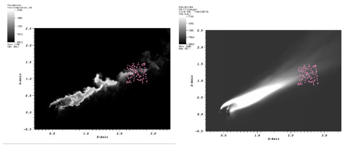
**Figure 6:** Instantaneous (left) and time-averaged (right) temperature plots with the PFTIR instrument model target samples shown with pink markers.
