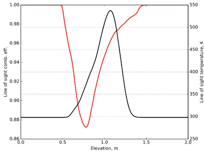
**Figure 4:** Combustion efficiency (red line) and temperature (black line) line of sight LES predictions at a location downstream from the flare.
