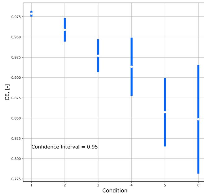
**Figure 9:** A plot of the 95% confidence interval from the raw measured data used to represent the relative variations in the combustion efficiency per case. The mean values are shown with the white dots.
