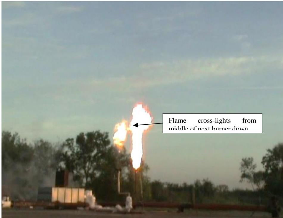
**Figure 3 - Multi-point flare cross lighting relies on hot-combustion gases (radicals) from the piloted burner to ignite the neighboring burner**
