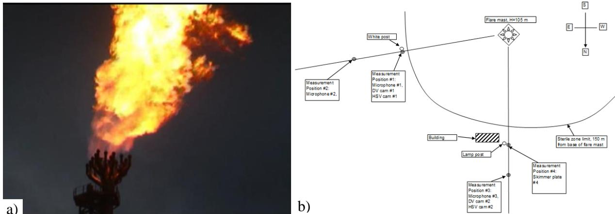
**Figure 5 - Elevated Multi-point flare: a) fireball generated during ignition process, b) experimental setup to measure pressure wave generated during the ignition process**
