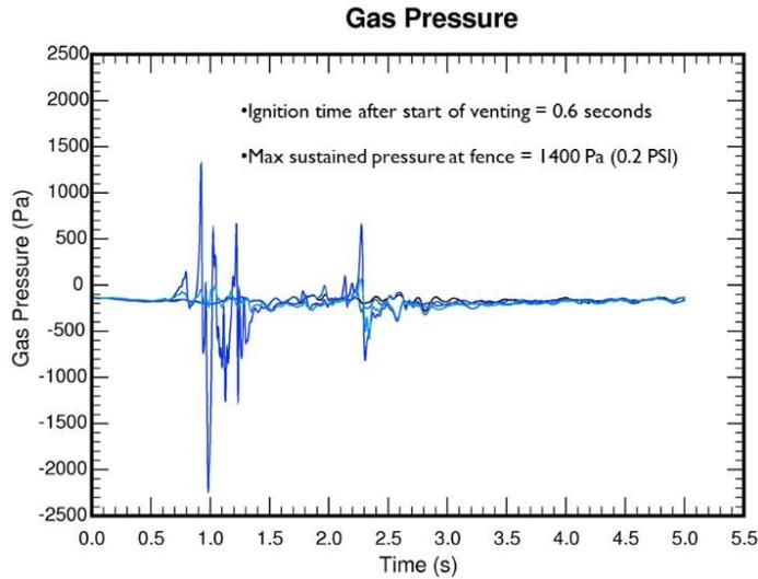
Figure 14 - Pressure wave generated during a MPGF ignition with a 150 ms delay
