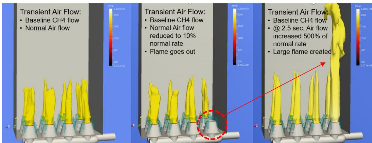
Figure 18 - Transient air flow fed to process burner can create overpressure condition in heater
