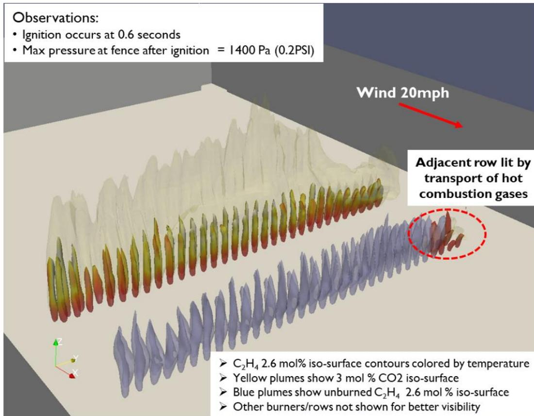
Figure 13 - MPGF ignition test with perpendicular cross wind blowing at 20mph from lit row to unlit row
