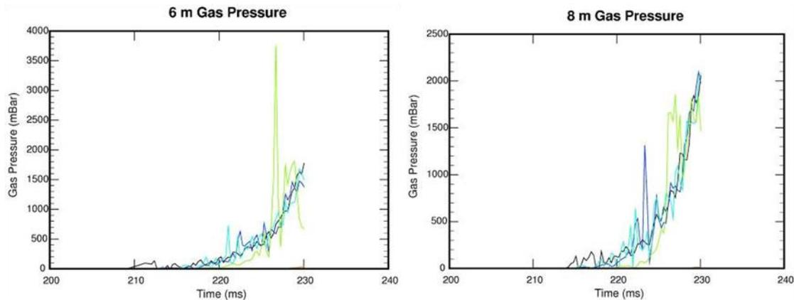
Figure 8 - Pressure around an elevated multi-tip flare with a 250 ms ignition delay
