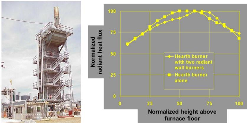
Figure 19 - Heat flux profiles in a pyrolysis furnace with and without wall burners [16]
