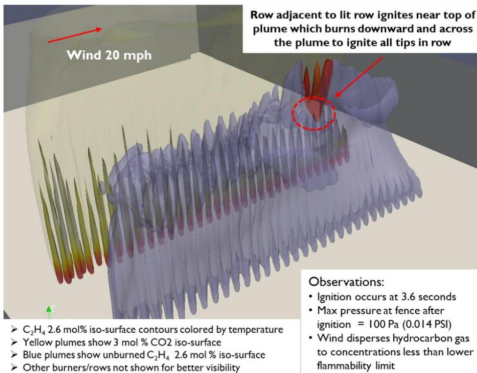
Figure 15- MPGF ignition test with 20mph parallel cross wind
