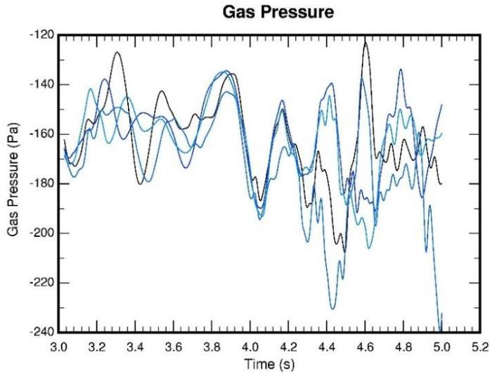
Figure 16 - Pressure wave created with ignition under a 20mph wind blowing parallel to the lit row
