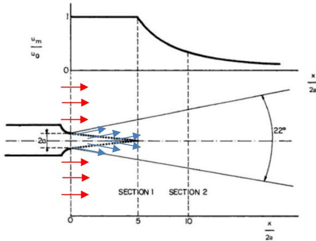
Figure 6 – Use of a free jet discharging into a calm atmosphere – the region outlined by dots is a constant velocity cone which extends 5 nozzle diameters. This approximation was used in length.
