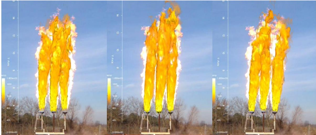
Figure 4 - Comparison of predicted and measured flame shape for a 3-Flare Test burning ethylene gas [15]
