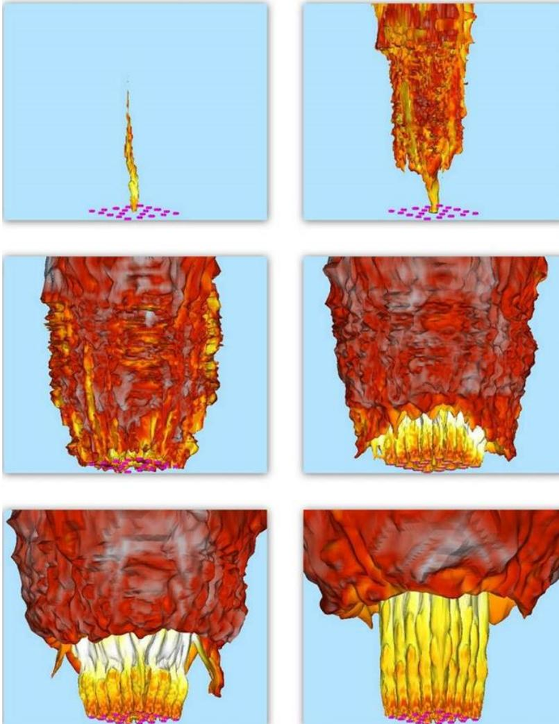
**Figure 7 - Growing fireball during elevated flare ignition with 250 ms ignition delay**
