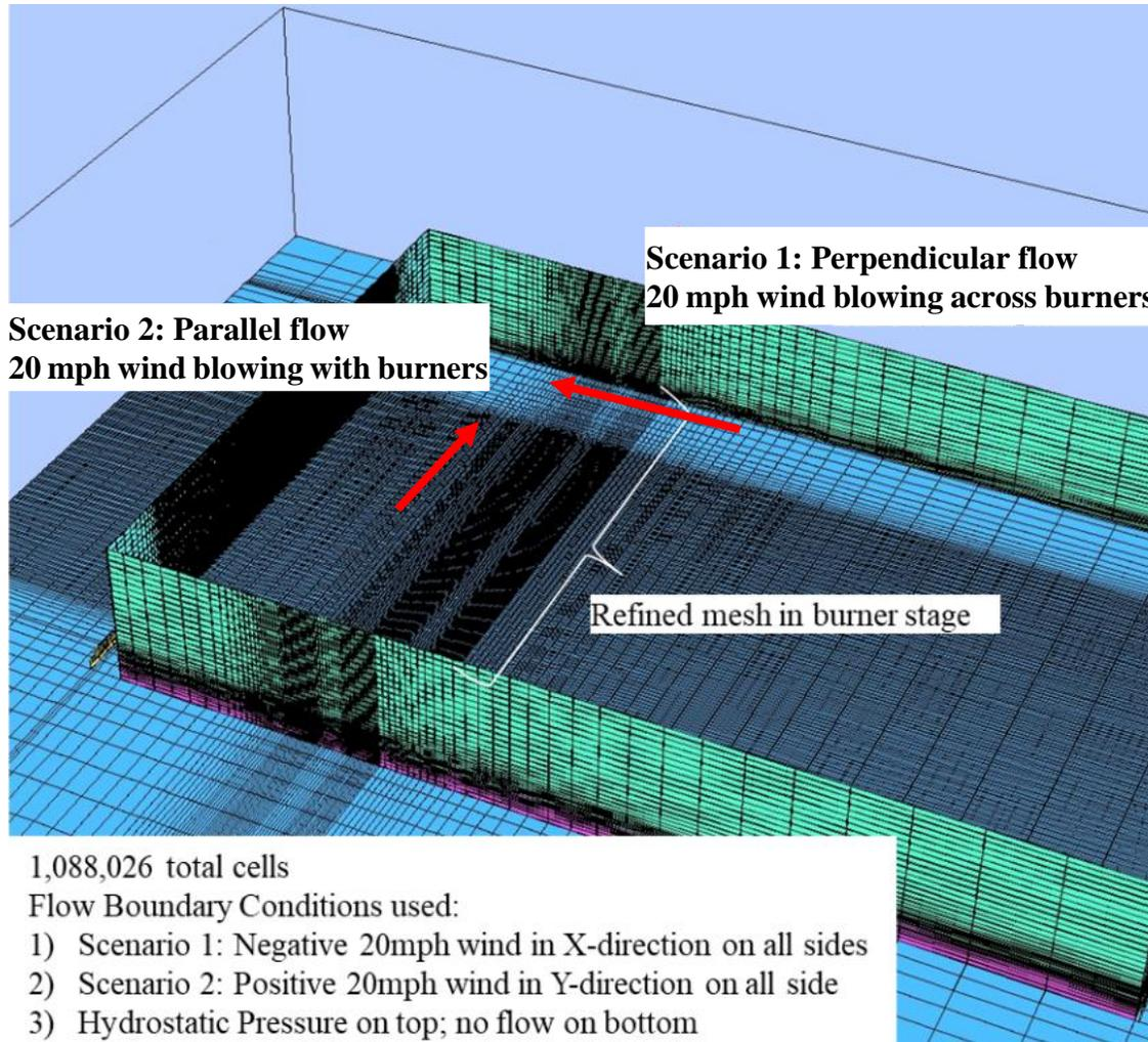
Figure 12 - Computational mesh of Ethylene flare with boundary conditions
