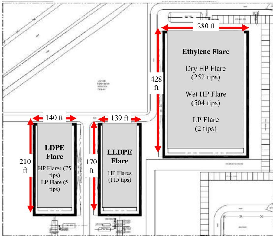
Figure 10 - Plan view of multi-field MPGF showing ethylene field and structures included in CFD analysis
