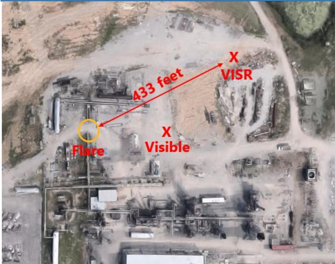
**Figure 3: Approximate position of flare, VISR imager and visible camera**
