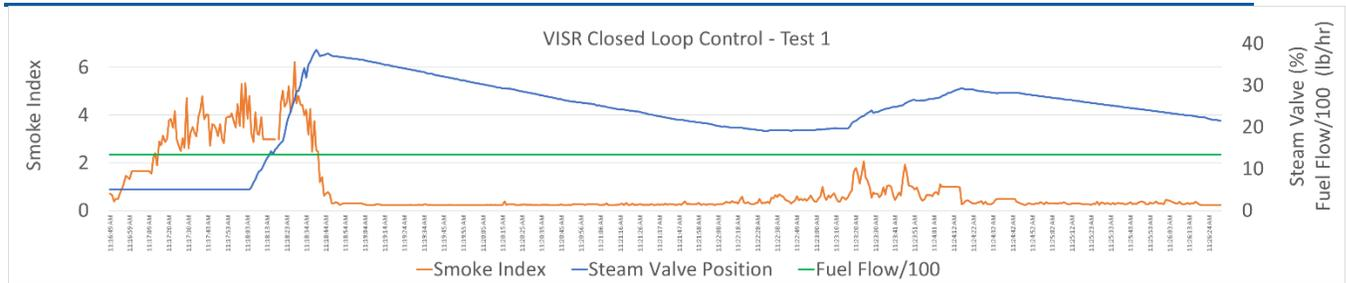
Figure 5: Time series plot of SI, Steam Valve Position and Fuel Flow rate for Test 1
