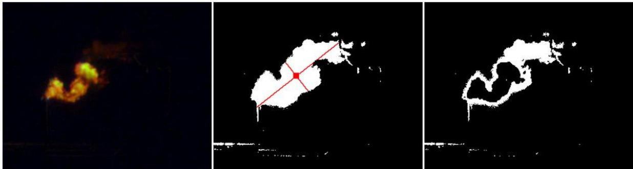
**Figure 1: VISR spectral image (left), flare footprint (center) and combustion envelope (right).**
