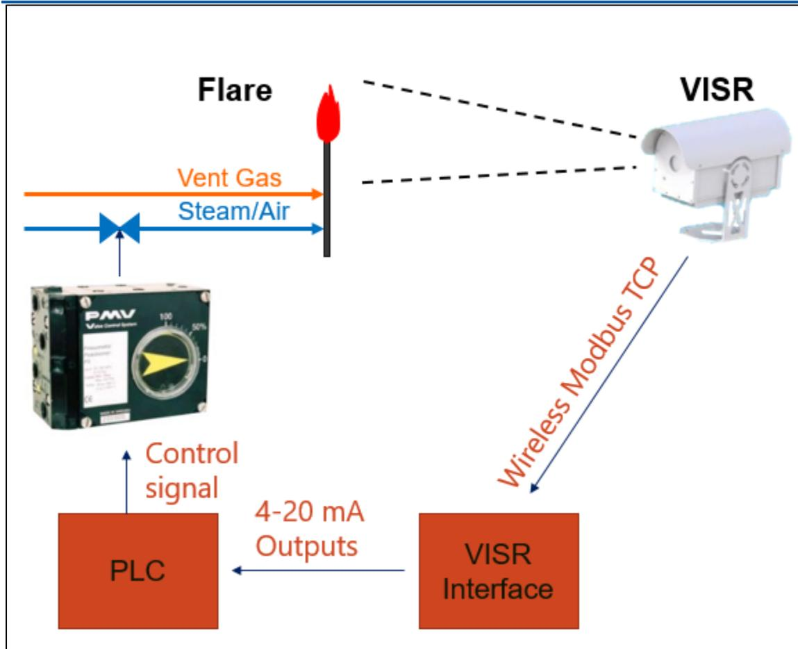
Figure 4: Configuration of equipment for closed loop control.
