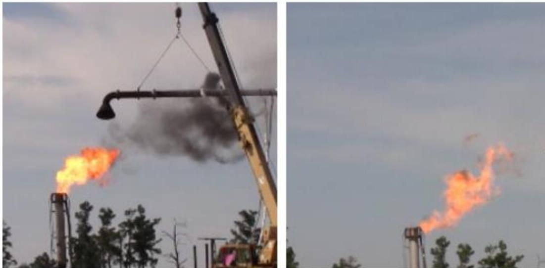
Figure 2: Flare with SI = 5.6 (left) and SI = 1.5 (right)
