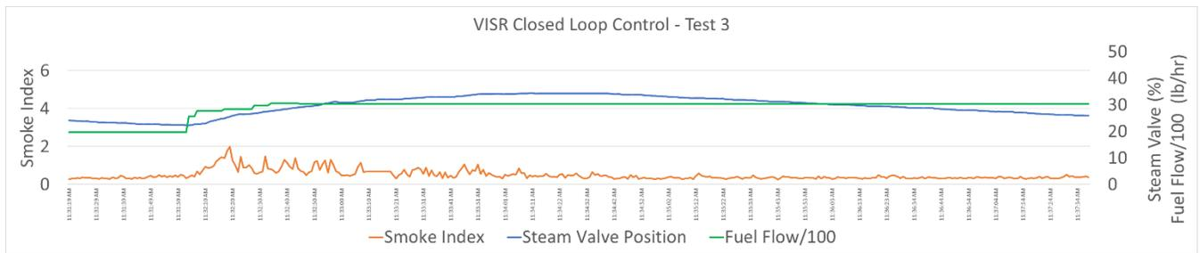
Figure 7: Time series plot of SI, Steam Valve Position and Fuel Flow rate for Test 3
