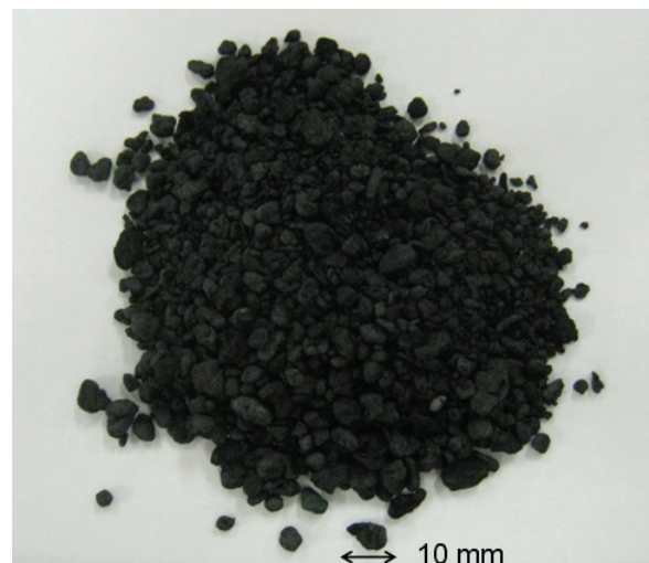
Fig. 2 Photo of sewage sludge after carbonization
