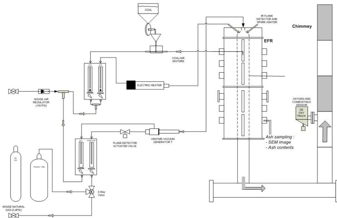
**Figure 2 - Schematic Diagram of Entrained Flow Reactor [7]**
