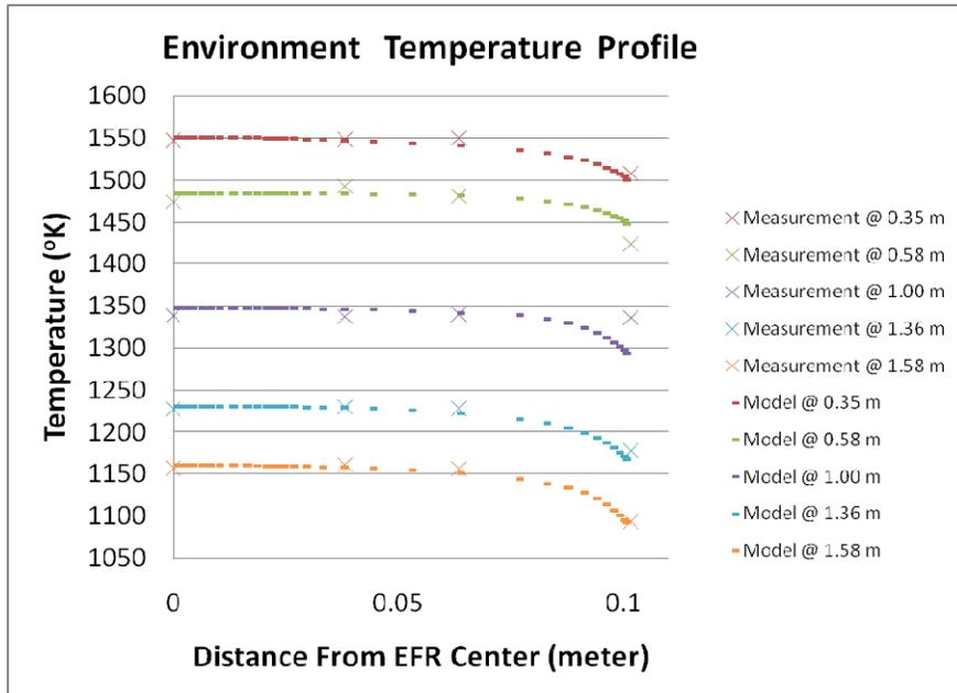
Figure 3 - Temperature profile across the EFR during coal combustion.
