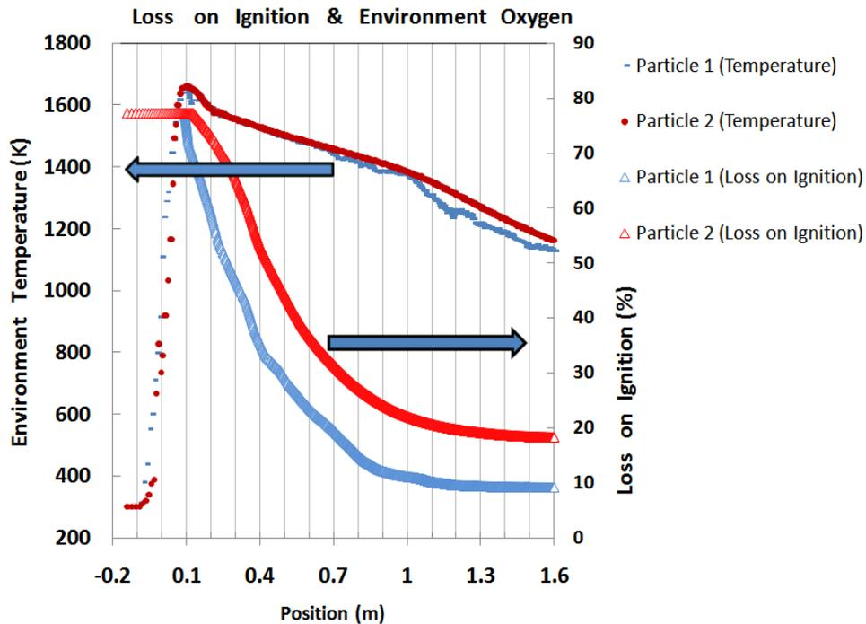
**Figure 6 - Environment temperature history and loss on Ignition computed by Fluent embedded CBK model for two 110um.**
