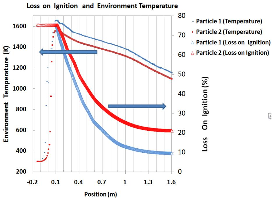
Figure 8 - Temperature history and % Loss on Ignition computed by CBK for two 110um particles
