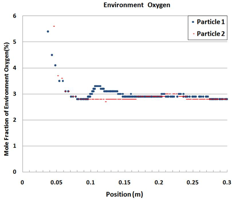
**Figure 5 - Oxygen concentration paths of two 110 um particles with similar temperature**
