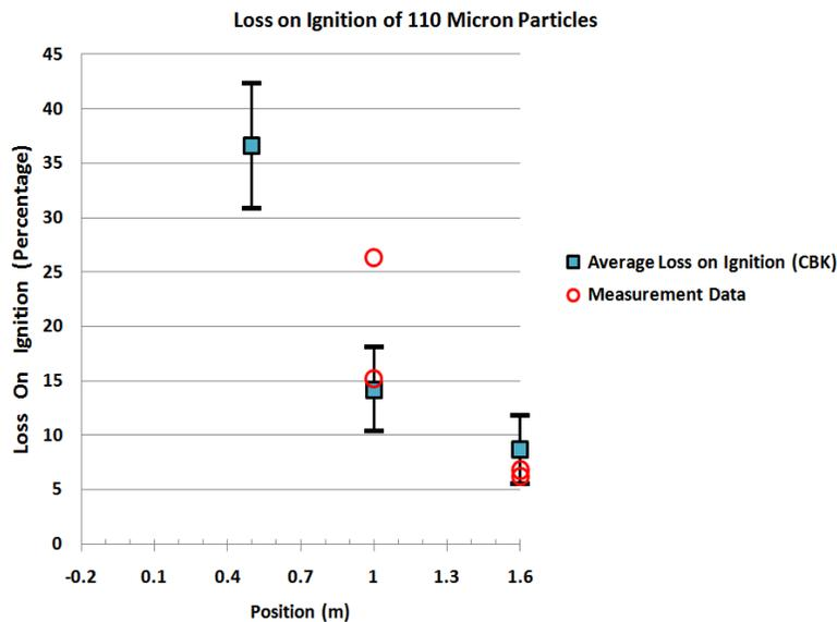
**Figure 9 - Measured Loss on Ignition and average Loss on Ignition predicted by CBK model for 110 micron particles**
