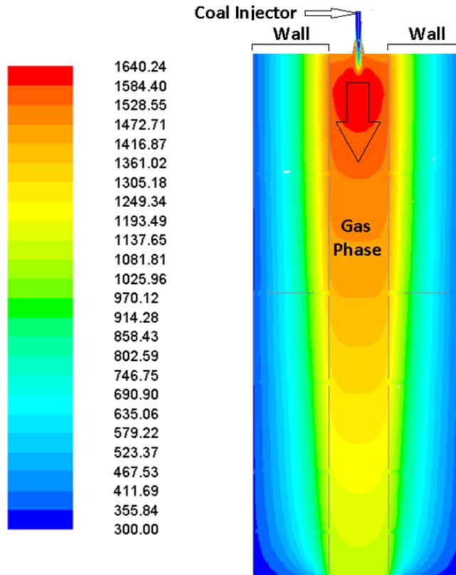
**Figure 4 - Fluent simulation predicting static temperature including gas phase and solid phase during Eastern Bituminous coal test.**
