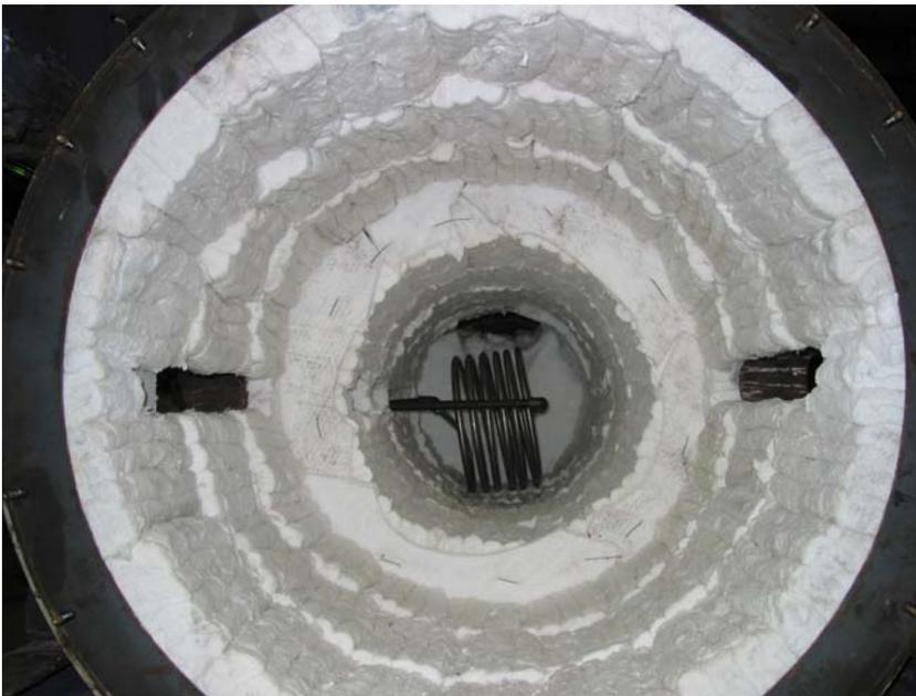
Figure 3: The inside of the RTF showing the insulation and the heat transfer coil just before the wall.
