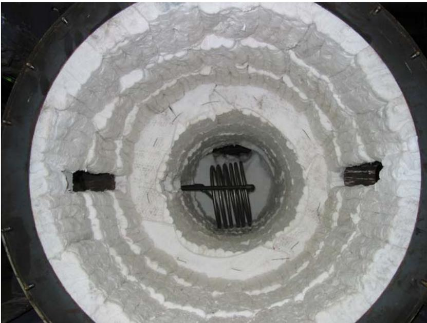
Figure 3: The inside of the RTF showing the insulation and the heat transfer coil just before the wall.
