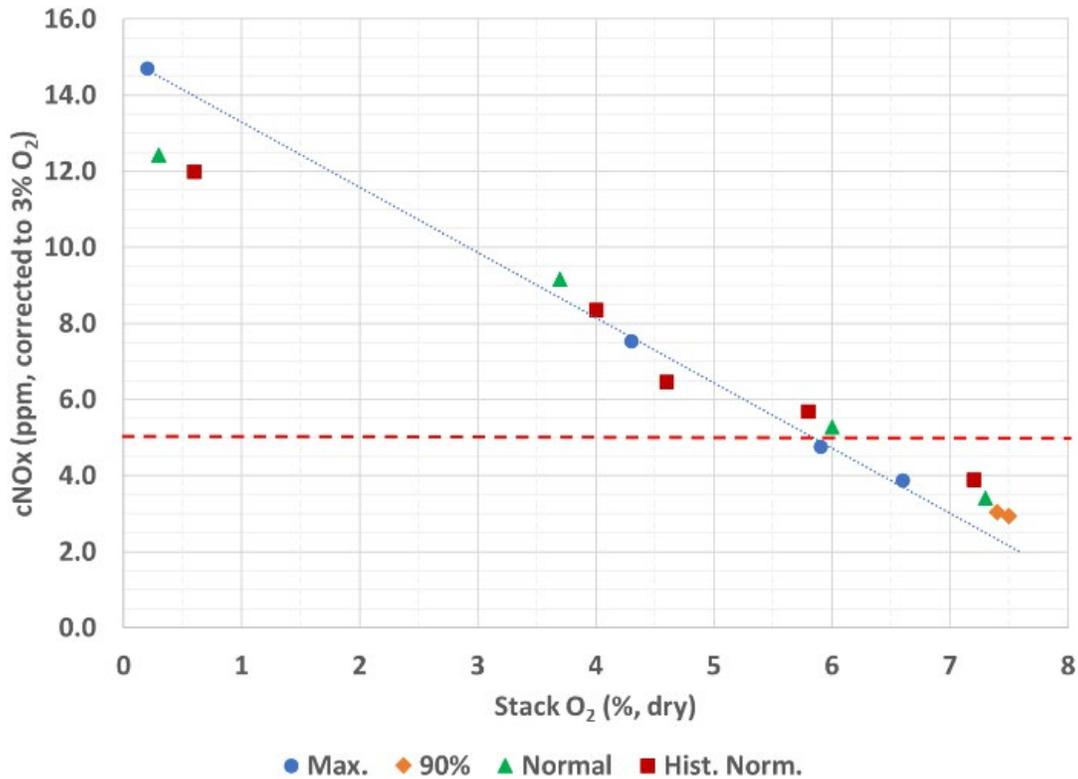
Figure 5 - Stack oxygen versus corrected NO<sub>x</sub> for Heater 1.
