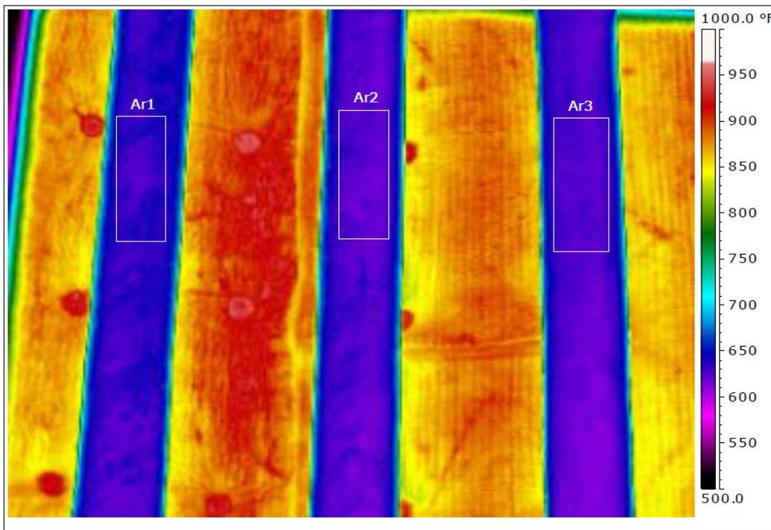
**Figure 8 - Infrared (IR) scans of the process tubes in the heater.**
