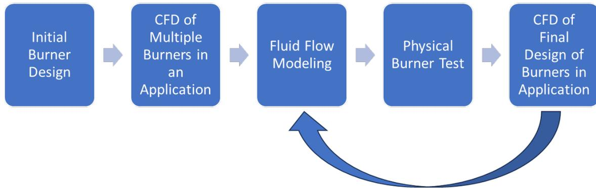
**Figure 2 - Flow chart of ClearSign Core burner project design scenario timeline.**
