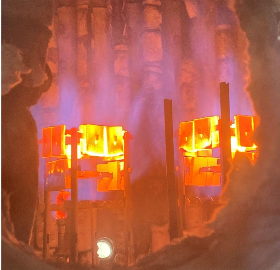
**Figure 7 - Multi-burner configuration, showing the flame holder portion of the burner, within the furnace.**
