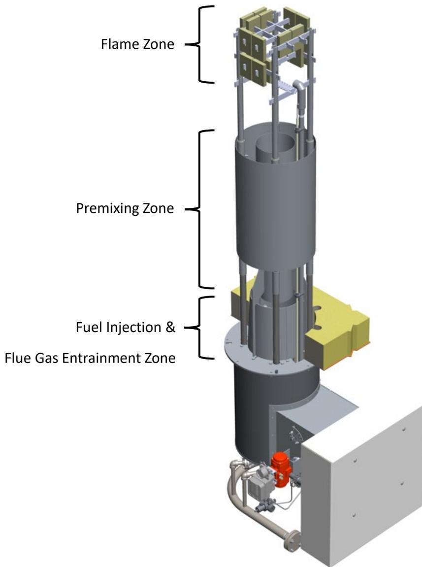
**Figure 1 - Schematic of ClearSign Core™ Natural Draft Process Burner**
