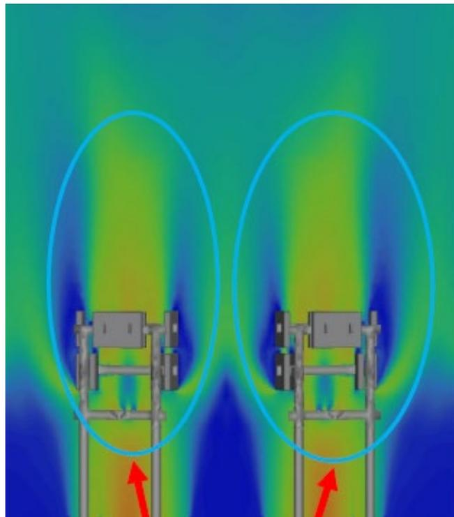
**Figure 4 - By reducing the width of the flame anchor and eliminating internal tiles, the flow was successfully redirected axially.**
