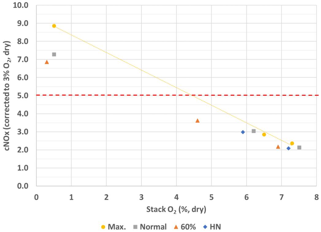
**Figure 6 - Stack oxygen versus corrected NO<sub>x</sub> for Heater 2.**
