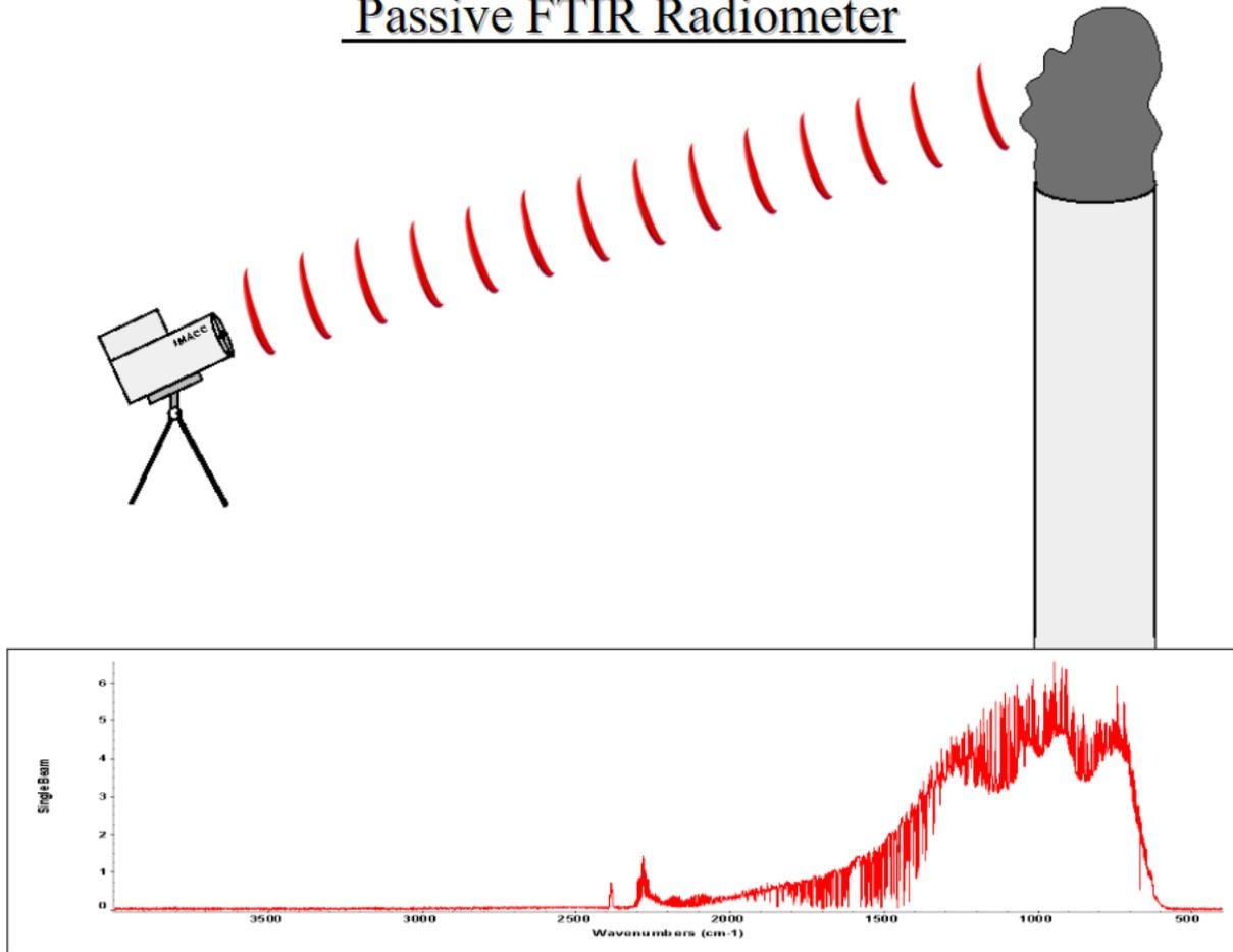
Figure 4. Illustration of PFTIR for Flare Emissions Measurements.
