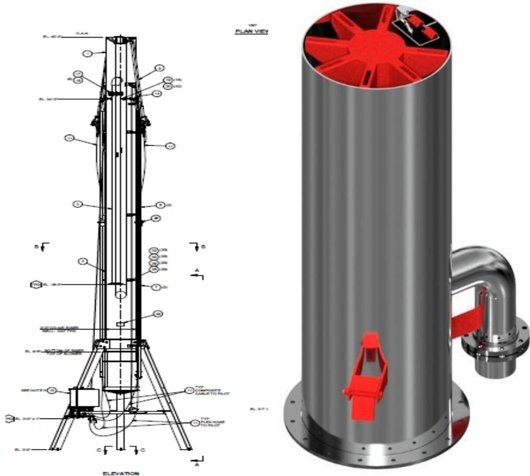
Figure 1. A conventional SFVP-0824x40 ft air assisted flare with fixed outlet areas offered by Cimarron. The center gas riser is for HP gas (connected to the red outlet spider nozzle). The riser hanging on the outside is for LP gas (connected to rectangular outlet). The air duct connected to the stack riser is supported by a tripod structure.
