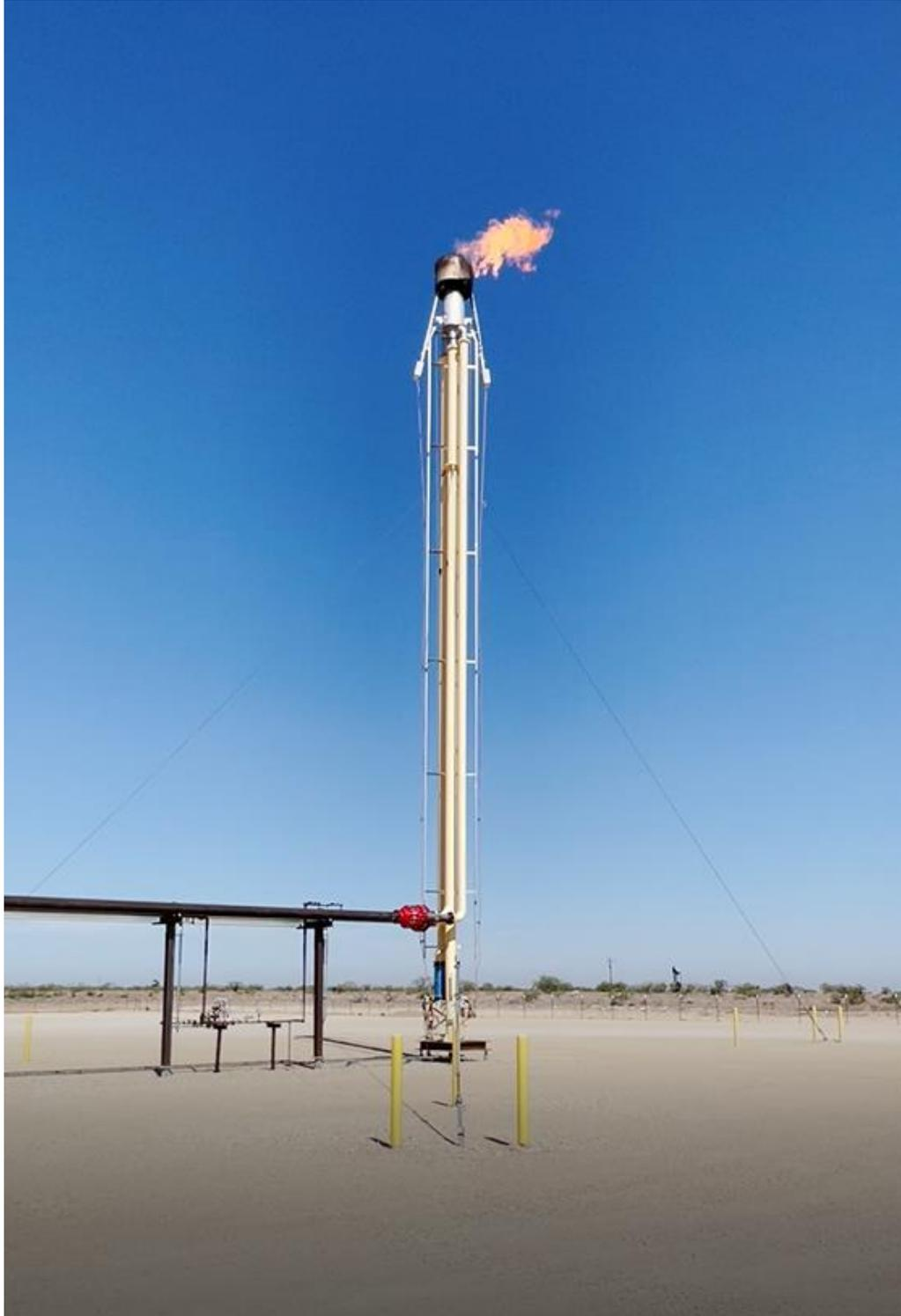
Figure 5. DreamDuo Flare Firing 130 MSCFD of LP gas.
