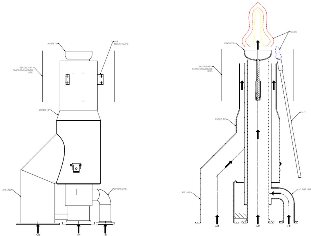
Figure 2. Cimarron's Patented DreamDuo Air Assisted Flare
