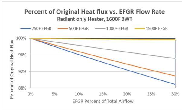
Figure 8: Radiant box heat flux comparison with various EFGR temperatures.
