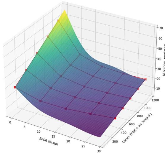
Figure 7: 3D plot of simulated  $\text{NO}_x$  reduction vs. EFGR flow and combustion air mix temperature for the 90% TNG/10  $\text{H}_2$  fuel mix.
