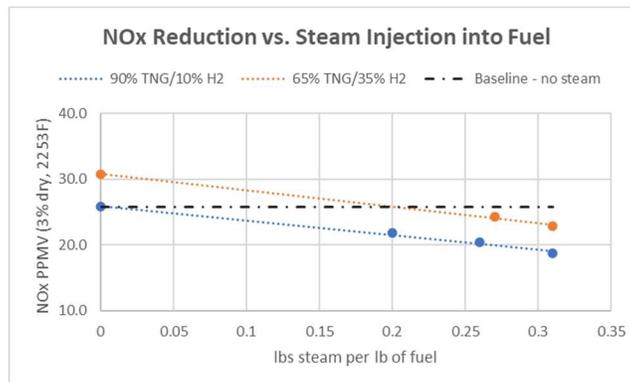
Figure 4: Steam injection test data, high peak firebox temperatures.
