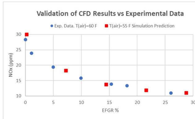
Figure 6: Plot showing a comparison of NO<sub>x</sub> values of experimental data against predicted CFD simulation values for similar conditions of EFGR flow, EFGR temperature, and combustion air temperature. Results are for the 90% TNG/10% H<sub>2</sub> fuel mix.
