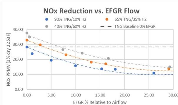
Figure 2: High EFGR temperature test data.
