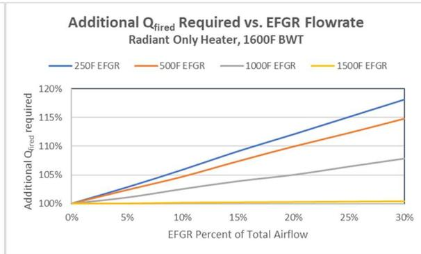
Figure 9: Additional heat input required to restore heat flux at various EFGR temperatures.
