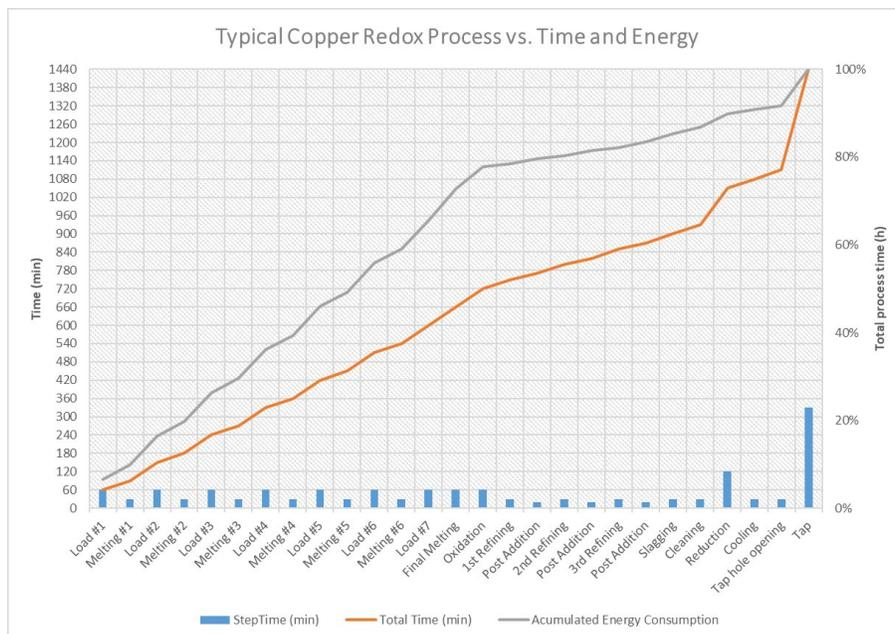
Figure 4. Common steps and for secondary copper recovery.
