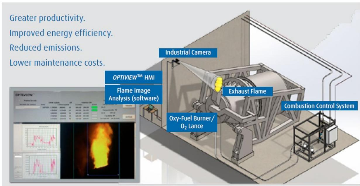
Figure 15. Typical OPTIVIEW installation and layout as developed for Tilting Rotary Furnaces.
