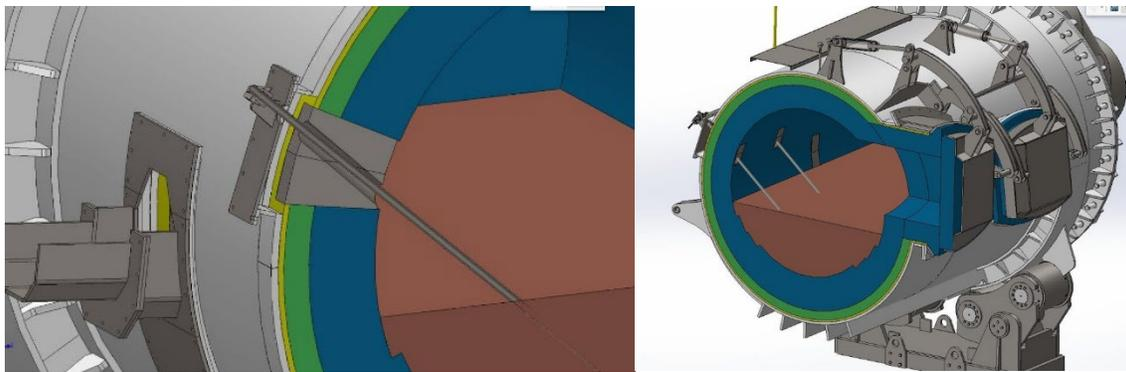
Figure 5. Model to simulate lancing step into a copper scrap furnace.
