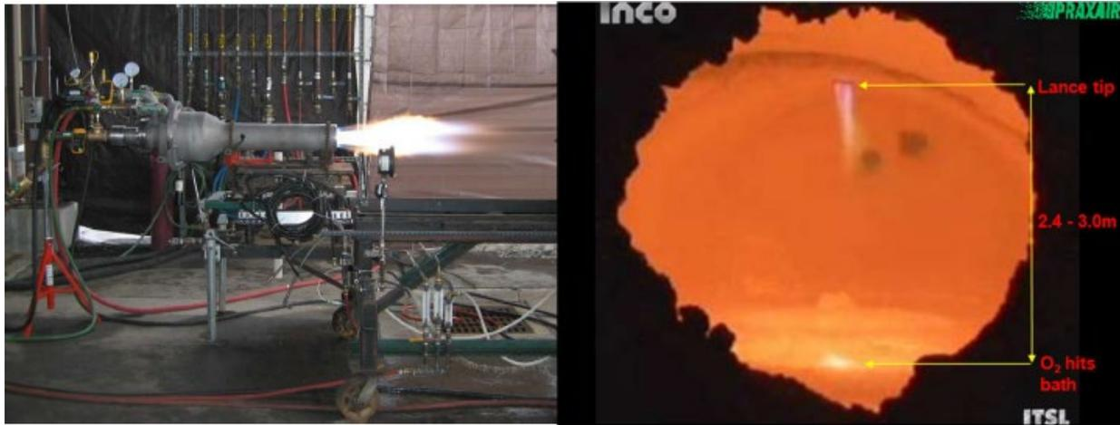
Figure 19. CoJet for copper been tested at Linde Technology facility in Tonawanda and in operation at Copper Furnace (Inco's MK Reactor) [10].
