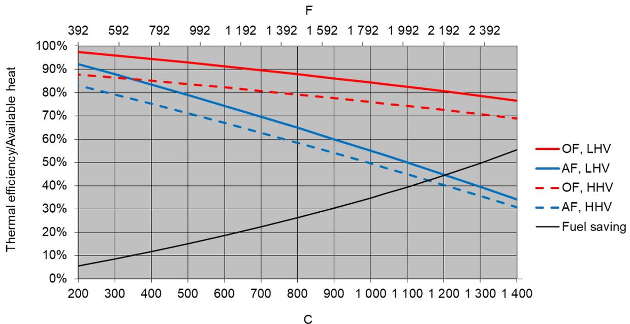
Figure 6. Thermal efficiency for Air-fuel and Oxy-fuel for different flue gas temperatures.
