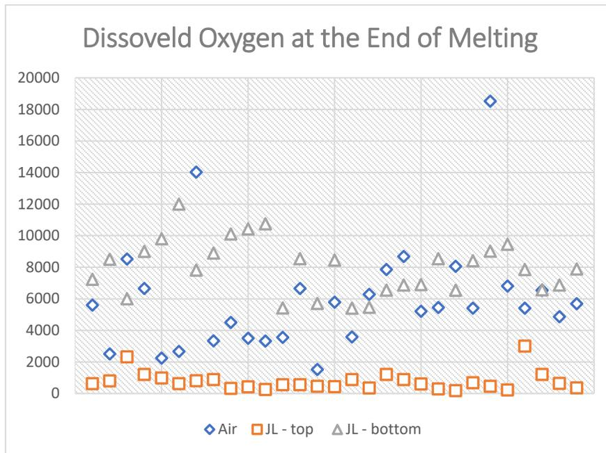
Figure 14. Different dissolved oxygen using Air-fuel, Oxy-fuel (JL-Lance on top), (JL – Lance on bottom)
