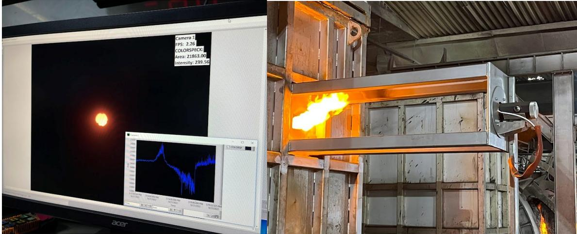
Figure 16. OPTIVIEW™ operation screen (left) and installation at copper furnace gas ends (right).
