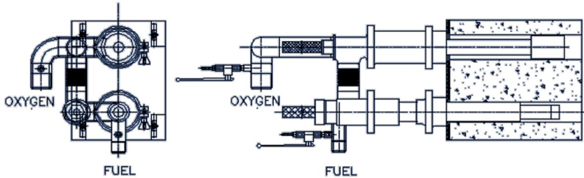
Figure 11. Typical design for a JL burner with lance on top (block with 11 x 16 in or 270 x 400 mm)
