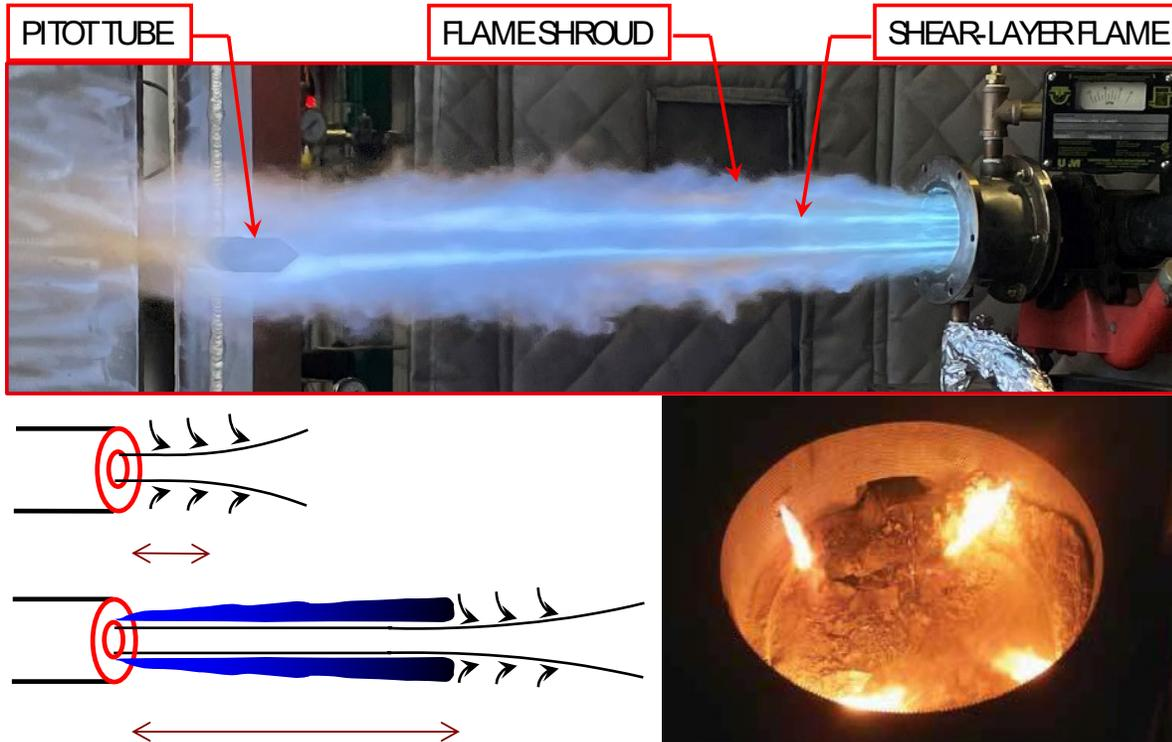
Figure 18. Top – O<sub>2</sub> *CoJet*<sup>®</sup> technology firing natural gas; Bottom Left – flame shrouding concept; Bottom Right – 165T DC EAF [10].
