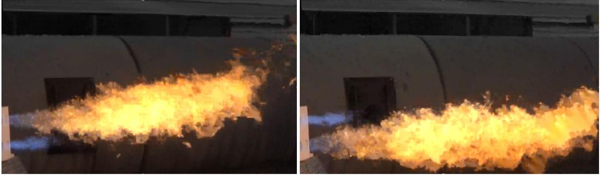
Figure 13. 7 MMBtu/h (2MW) flame with flexible JL (left: Lance on bottom, right: Lance on top).
