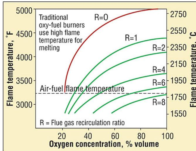
Figure 9. Flame peak temperature using Natural Gas for different recirculation ratios [7].
