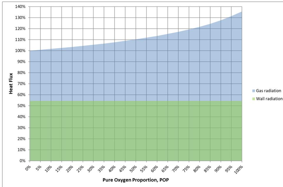
Figure 7. Heat transfer changes by radiation in function of different oxygen content as oxidant [6].
