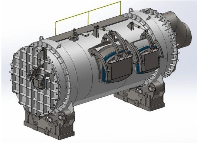
Figure 3. Typical design for Scrap Melting and Refining using TBBS.
