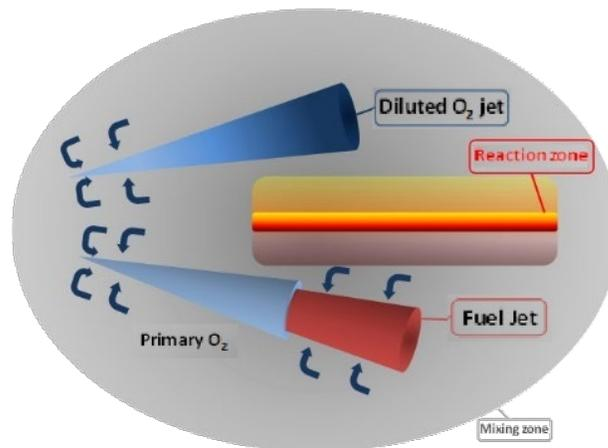
Figure 10. JL's flame profile with 2 different zones (fuel rich and oxygen rich).
