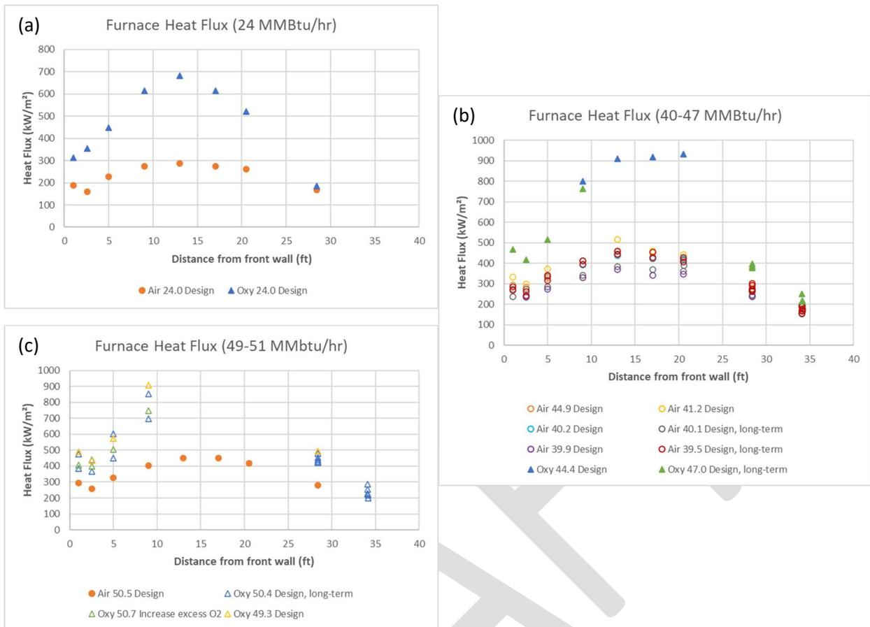
Figure 8. Furnace heat flux comparing air- and oxy-firing under various loads
