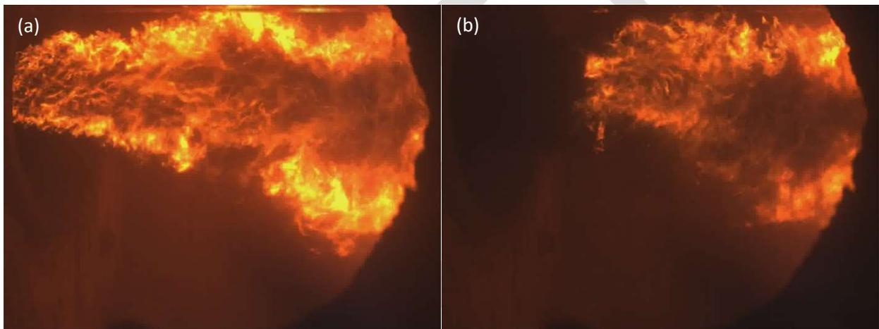
Figure 5. Oxy-fired flame under extreme off-design conditions (48 MMBtu/hr)
