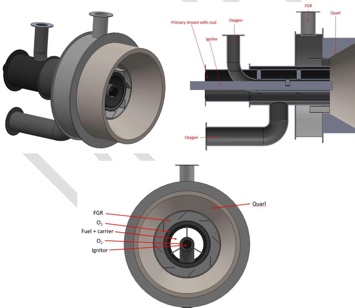
Figure 1. JOC Annular Shroud High-temperature Oxy-burner
