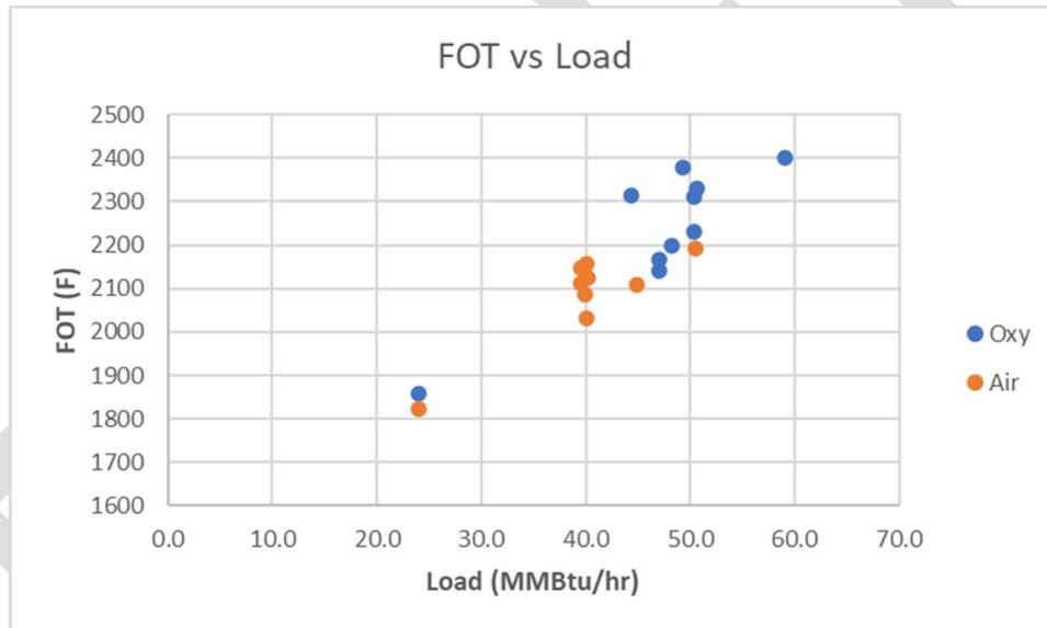
Figure 7. Furnace outlet temperature (FOT) as a function of load
