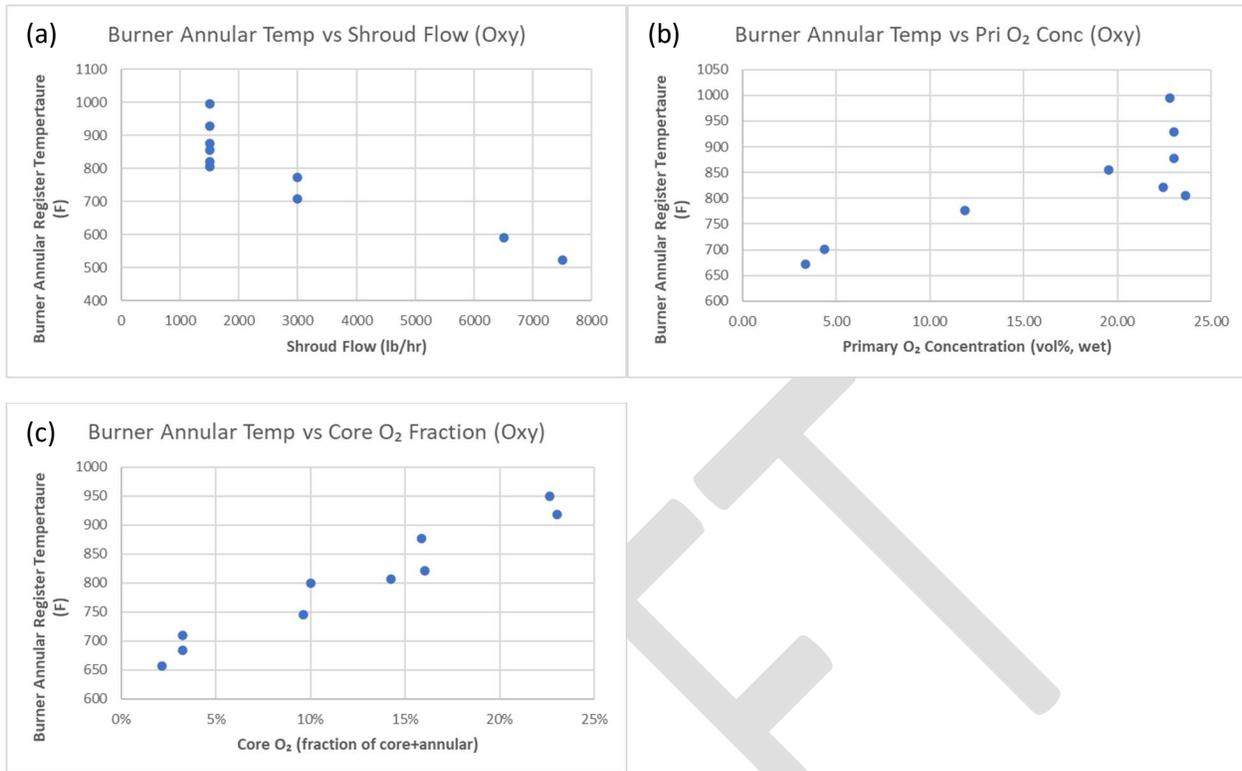
Figure 9. Burner annular register metal temperature as a function of (a) shroud flow, (b) primary oxygen concentration, and (c) fraction of oxygen to the core under oxy-fired conditions
