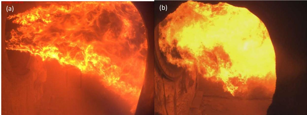
Figure 4. Flame images at design conditions (a) oxy-fired at 59 MMBtu/hr, (b) air-fired at 51 MMBtu/hr
