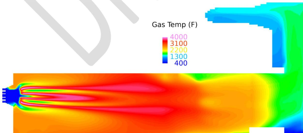
Figure 11. Oxy-fired 59 MMBtu/hr CFD model prediction of gas temperature
