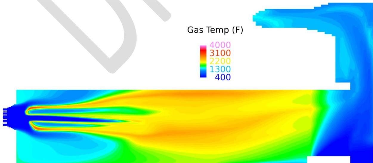
Figure 14. Air-fired 48 MMBtu/hr CFD model prediction of gas temperature
