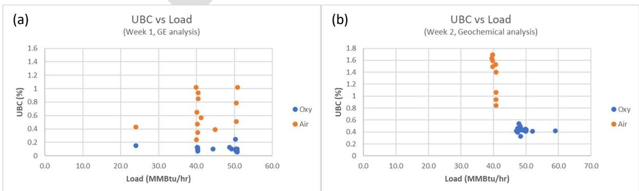
Figure 6. UBC in fly ash as a function of load
