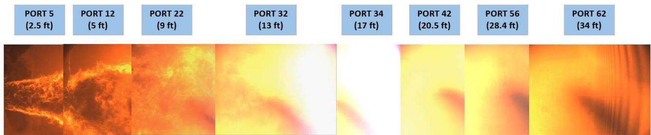
Figure 12. Oxy-fired 59 MMBtu/hr camera images
