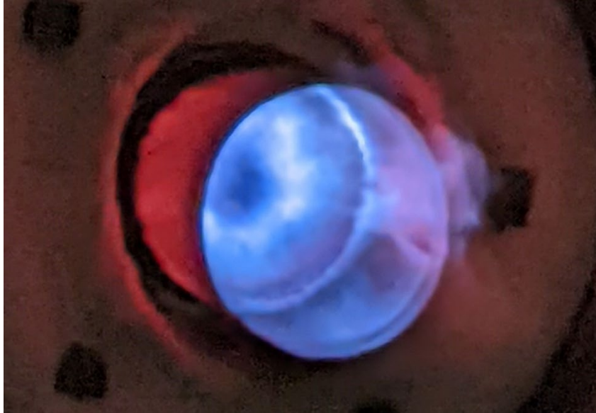
Figure 3. Nozzle Mix Burner-75% Hydrogen 25% Natural Gas at 0.500 MMBtu/hr with 46% Excess Air
