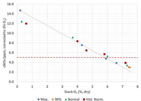
Figure 5 - Stack oxygen versus corrected NO<sub>x</sub> for Heater 1.
