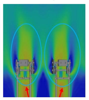
Figure 4 - By reducing the width of the flame anchor and eliminating internal tiles, the flow was successfully redirected axially.
