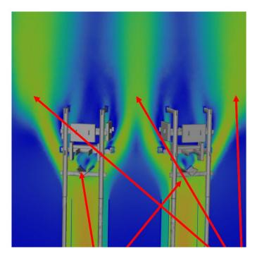
Figure 3 - The initial flame anchoring points, located at the base of the flame holder, led to flow diversion, and created the potential of flames merging.
