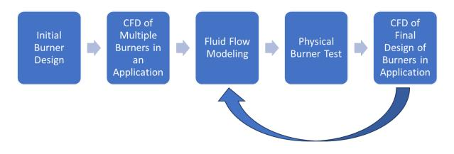
Figure 2 - Flow chart of ClearSign Core burner project design scenario timeline.
