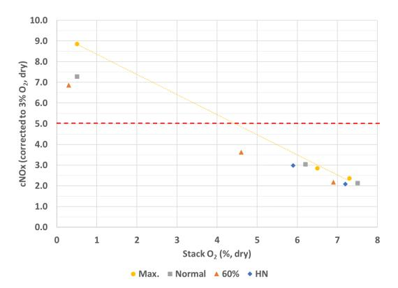
**Figure 6 - Stack oxygen versus corrected NO**<sub>x</sub> for Heater 2.
