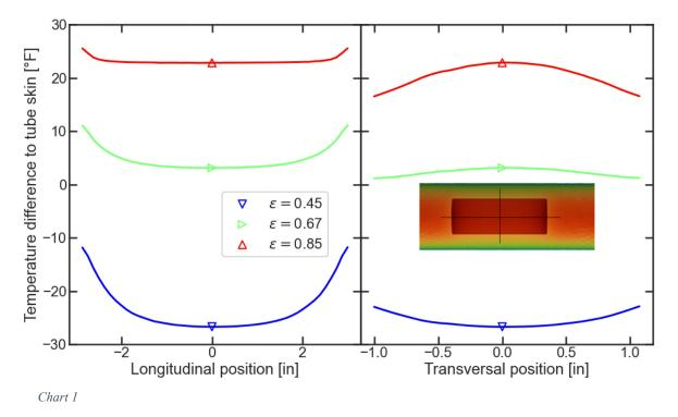
CFD simulation was done for high severity conditions to understand the impact of higher temperature on the butter-pad temperature as compared to the bare surface.
