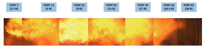
Figure 15. Air-fired 48 MMBtu/hr camera images
