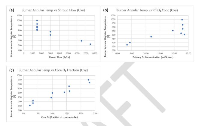
Figure 9. Burner annular register metal temperature as a function of (a) shroud flow, (b) primary oxygen concentration, and (c) fraction of oxygen to the core under oxy-fired conditions
