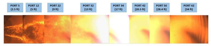
Figure 12. Oxy-fired 59 MMBtu/hr camera images
