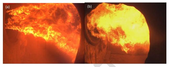
Figure 4. Flame images at design conditions (a) oxy-fired at 59 MMBtu/hr, (b) air-fired at 51 MMBtu/hr
