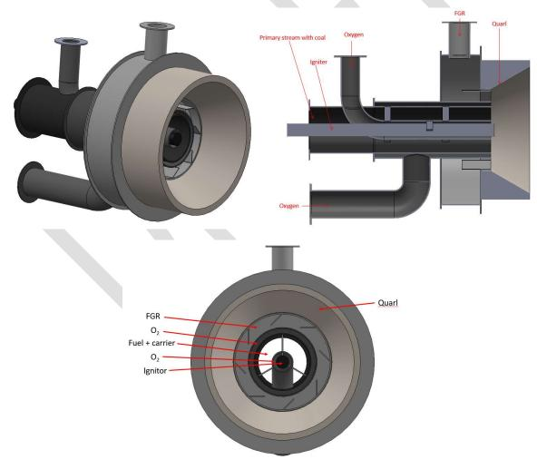
Figure 1. JOC Annular Shroud High-temperature Oxy-burner
