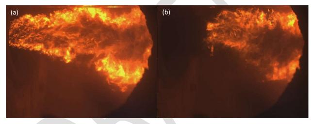
Figure 5. Oxy-fired flame under extreme off-design conditions (48 MMBtu/hr)
