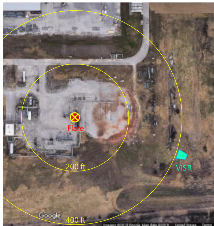
Figure 1: Site map showing the locations of the flare and the VISR device during the initial flare flow rate test.
