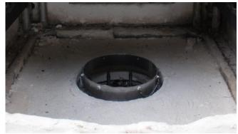
Figure 5 Generic burner EC Sensor electrode configuration.
