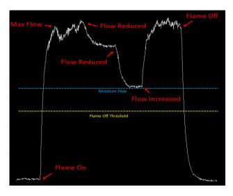
Figure 3 Flame On/Flame Off testing over a range of firing rates.
