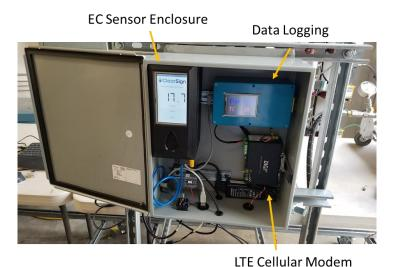
Figure 1 EC Sensor Electronics with data logging and remote monitoring for field installations.
