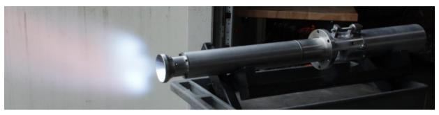
Figure 2 Test pilot burner designed with integrated EC Sensor.
