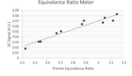
Figure 4 Calibration curve for equivalence ratio of burner.
