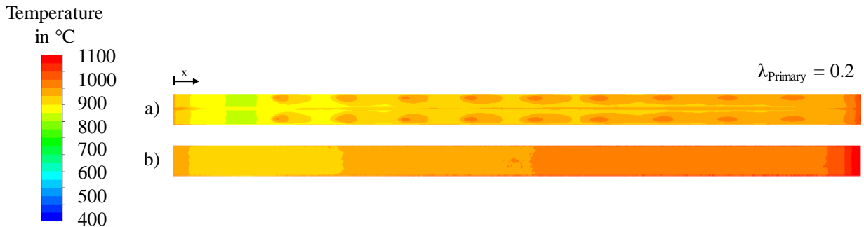
Figure 4: numerical temperature distribution on the radiant tube surface for \lambda_{\text{Primary}} = 0.2 a) 36 holes with \varnothing = 1.6 mm b) 72 holes with \varnothing = 1.2 mm
