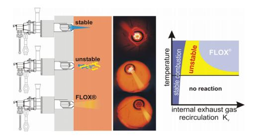
Figure 3: stable and unstable combustion
