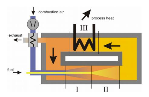
Figure 2: principle of Flameless Oxidation
