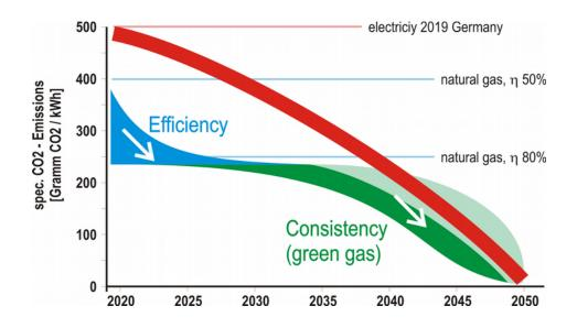
Figure 1: fossile CO2-emissions from high temperature process heating
