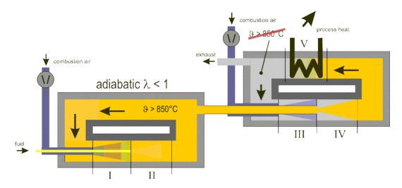
Figure 4: Two Stage Flameless Oxidation (FLOX®-2)
