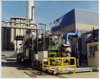
2-8 MW single burner test rig "CA.SPER."
