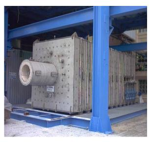
5 MW single burner test furnace "FO.SPER"
